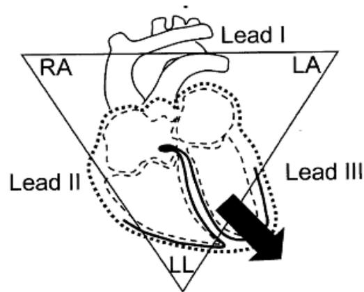
*Figure 5: Lead II configuration as represented by Einthoven's triangle superimposed on the cardiac conduction system and electrical dipole vector for the R wave of the ECG complex (Adapted and modified from Berntson et al, 2004)*
