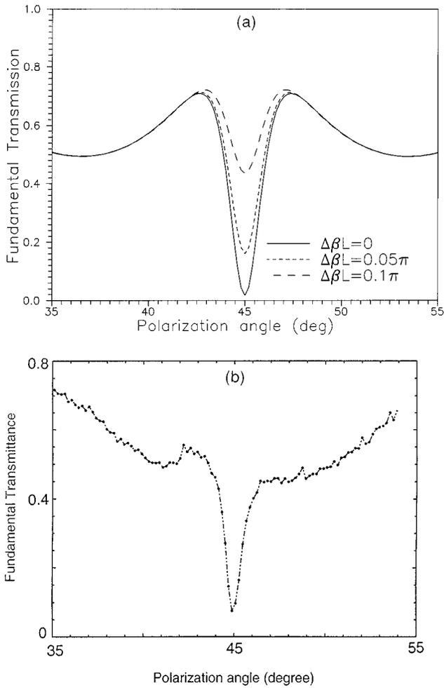
FIG. 2. Fundamental throughput  $\eta = (|A_1(L)|^2 + |A_2(L)|^2) / (|A_1(0)|^2 + |A_2(0)|^2)$  vs angle of polarization at the entrance facet of the crystal.  $45^\circ$  corresponds to balanced excitation, i.e., standard type II SHG. (a) Numerical calculation including time averaging over a Gaussian pulse and for various wave vector mismatches; (b) experimental results with 26 ps pulses.
