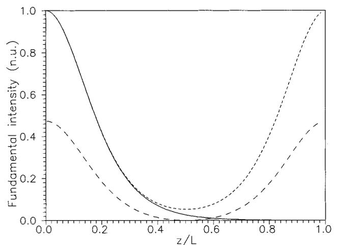
FIG. 1. Total normalized fundamental intensity  $\eta(z) = (|A_1(z)|^2 + |A_2(z)|^2) / (|A_1(0)|^2 + |A_2(0)|^2)$  vs distance  $z/L$  at phase matching for  $r = |A_2(0)|^2 / |A_1(0)|^2 = 1$  (solid line) and  $r = 0.9$  (short dashed). In the latter case the long-dashed line represents the weaker ( $|A_2(z)|^2$ ) component. Total input excitation was  $L^2 \chi^2 P = 25$  at  $\omega$ , and the calculation was carried out using plane waves and cw fields.
