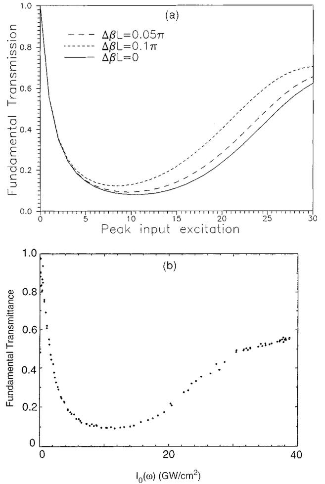
FIG. 3. Fundamental throughput  $\eta$  vs total FF input fluence for a fixed ratio  $r \approx 0.98$  between the FF components in  $z=0$ . (a) Numerical simulation for  $\Delta\beta L = 0, 0.05\pi, 0.1\pi$ , and time integration; (b) experimental results. A normalized excitation  $L^2\chi^2 P = 30$  corresponds to an intensity of 32  $\text{GW}/\text{cm}^2$ .
