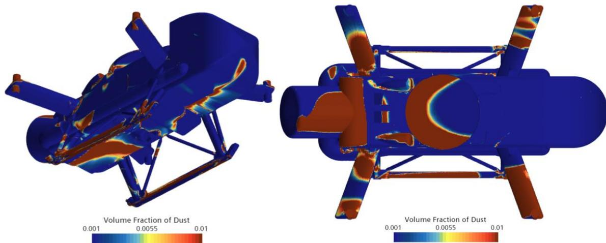
*Figure 13: Dispersed Multiphase Surface Volume Fraction Model*
