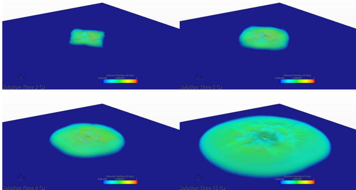
Figure 11: Unsteady Time Quadcopter Dust Cloud Formation
