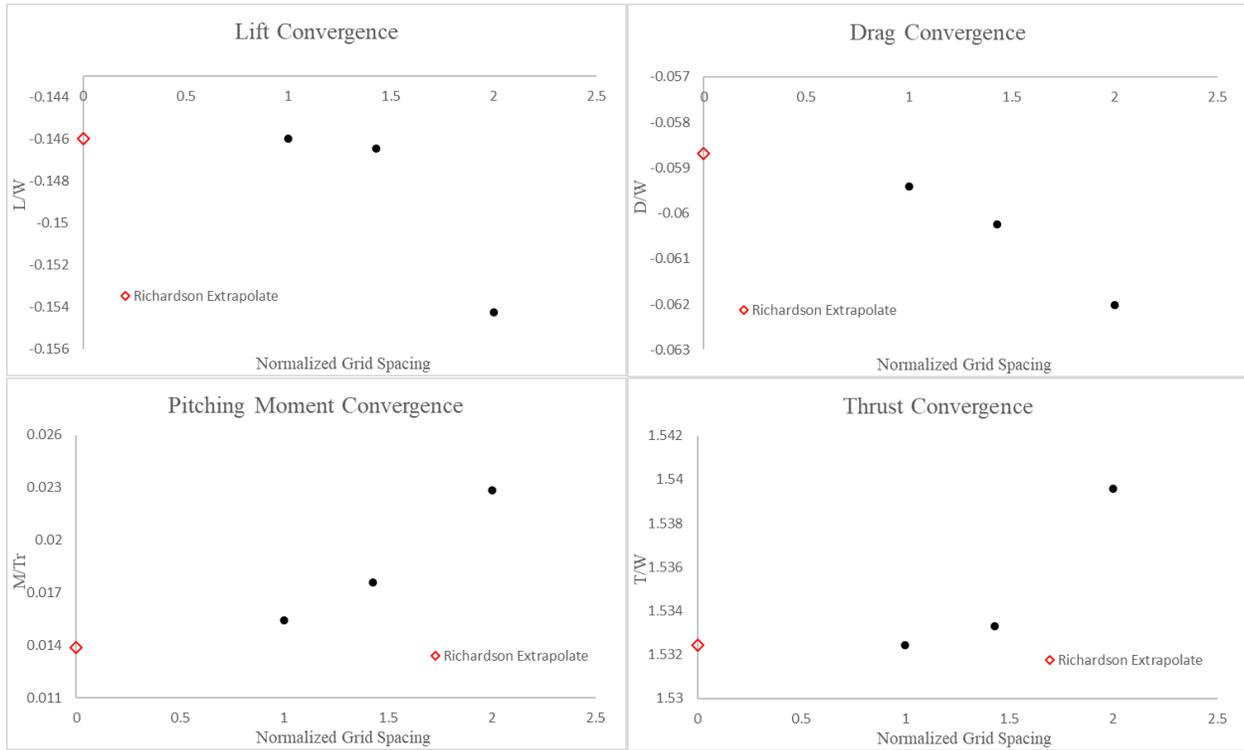
Figure 3: Grid Convergence Study of Aerodynamic Loads
