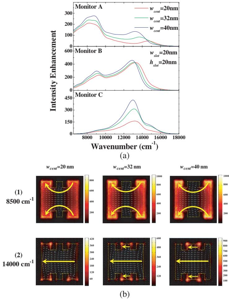
**Figure 8.** (a) Local intensity enhancement of the DS-DS MM for different monitor positions (see Fig. 2(b) for monitor locations). (b) The electric energy density of the DS-DS MM for the two plasmon resonances when  $w_{cent} = 20\text{ nm}$ ,  $32\text{ nm}$  and  $40\text{ nm}$ , respectively. The results are normalized relative to the incident  $E$ -field.
