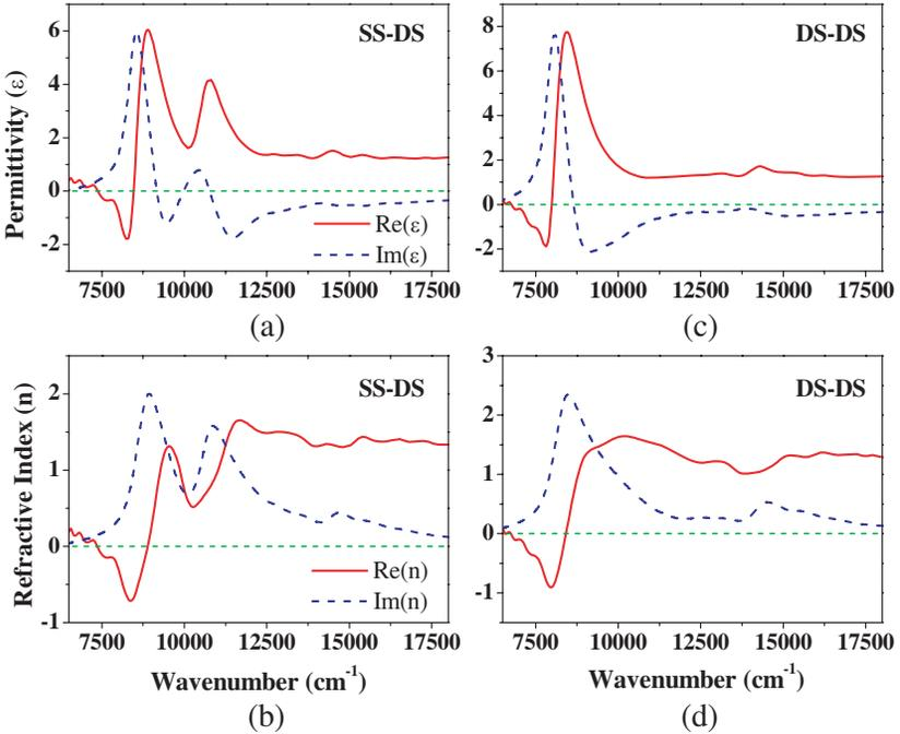
**Figure 5.** Extracted effective permittivity  $\varepsilon$  ((a) and (c)) and refractive index  $n$  ((b) and (d)) of the SS-DS and DS-DS.  $h_{slot} = 20 \text{ nm}$ ,  $w_{slot} = 20 \text{ nm}$ , and  $w_{cent} = 20 \text{ nm}$ , respectively.
