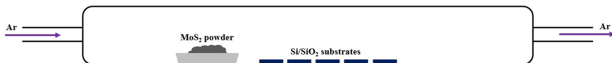
**Figure 1: Diagram of CVD setup**
