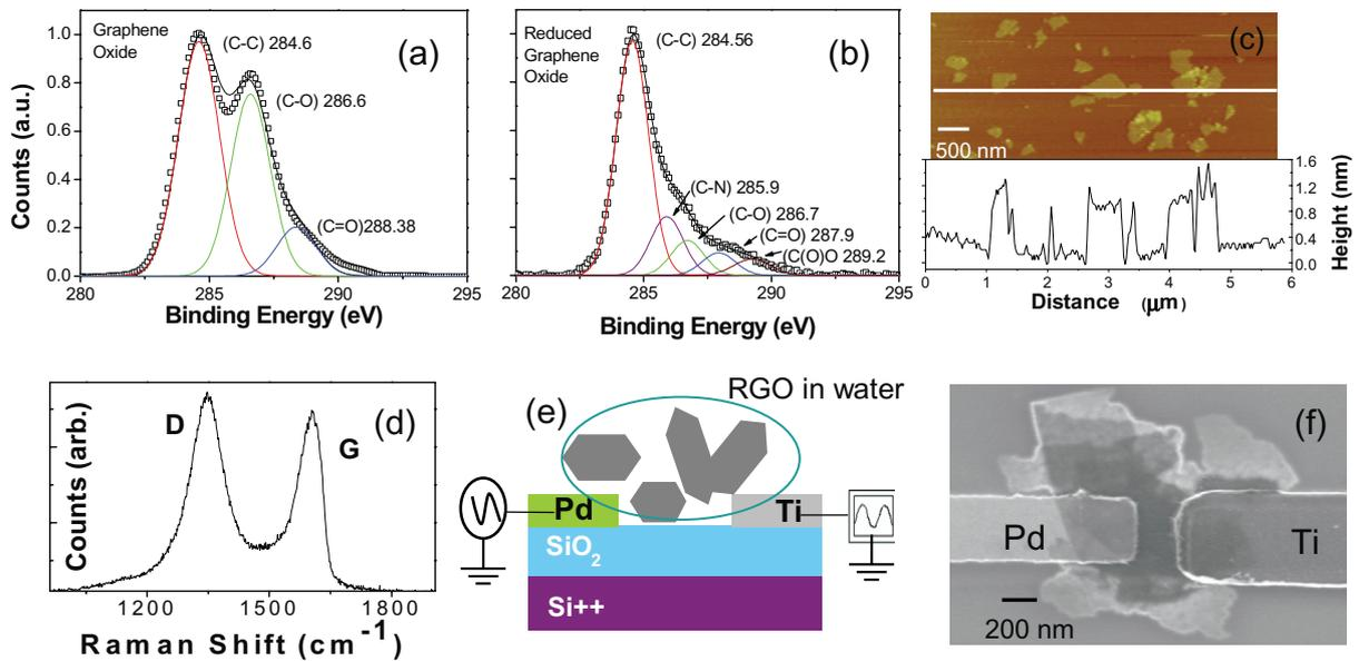
**Figure 1.** (a) XPS spectra of a GO thin film on Si/SiO<sub>2</sub> substrate. (b) XPS data for a RGO thin film. (c) Tapping-mode AFM image of RGO sheets with a height profile indicating that the majority of the sheets are single layer. (d) Raman spectra of RGO sheet. (e) Schematic diagram of the DEP assembly setup for RGO Schottky diode with Ti as Schottky and Pd as Ohmic contact. (f) SEM image of a DEP assembled RGO diode device.
