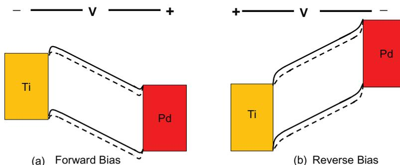
**Figure 4.** Energy band diagram of RGO Schottky diode before annealing (dashed line) and after annealing (solid line) under (a) forward and (b) reverse biased condition. A Schottky junction is formed between the RGO and Ti, and a bending of energy band occurs. After annealing, the work function of RGO increases, causing more bending at the Schottky contact.
