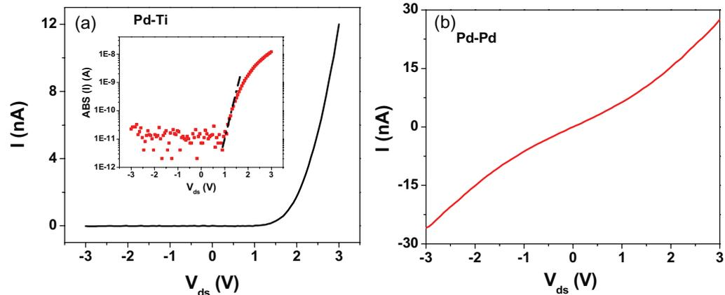
**Figure 2.** (a) A representative current–voltage ( $I$ – $V$ ) characteristics curve of a Ti/RGO/Pd Schottky diode assembled via DEP showing rectifying behavior. Inset: the semi-log plot of the absolute magnitude of current versus voltage of the device. The black line represents the linear fitting of the diode equation from which we obtain the ideality factor as  $n = 4.9$ . (b)  $I$ – $V$  curve of a control RGO device with Pd–Pd metal contact. No Schottky behavior can be seen.
