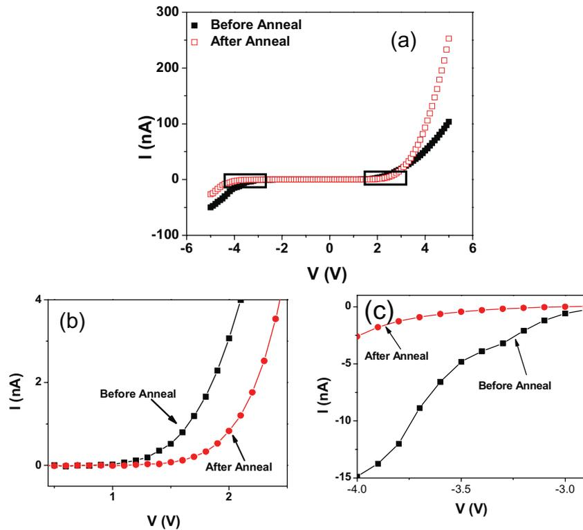
**Figure 3.** (a)  $I$ - $V$  curve of a RGO Schottky diode before and after annealing. (b) Magnified view of the  $I$ - $V$  characteristics in the forward biased regime, which show the turn-on voltage increased from  $1$  to  $1.5$  V upon annealing. (c) Magnified view of the  $I$ - $V$  curve in the reverse biased regime. The breakdown voltage changed from  $-3.1$  to  $-3.6$  V upon annealing.
