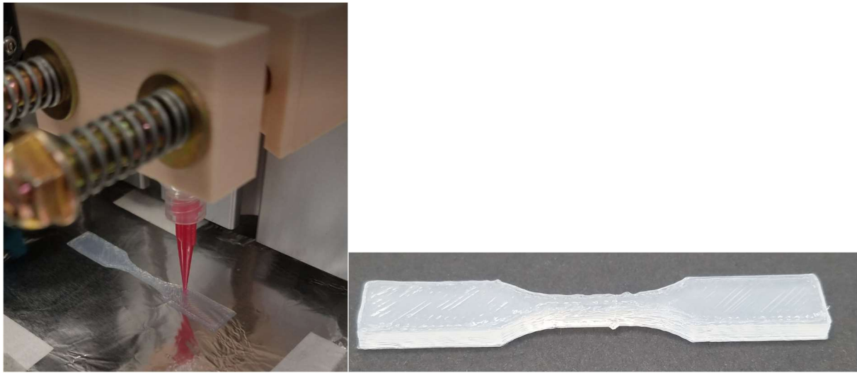
Figure 11: Tensile Beam During Printing (left), Fully Cured Tensile Beam (right)
