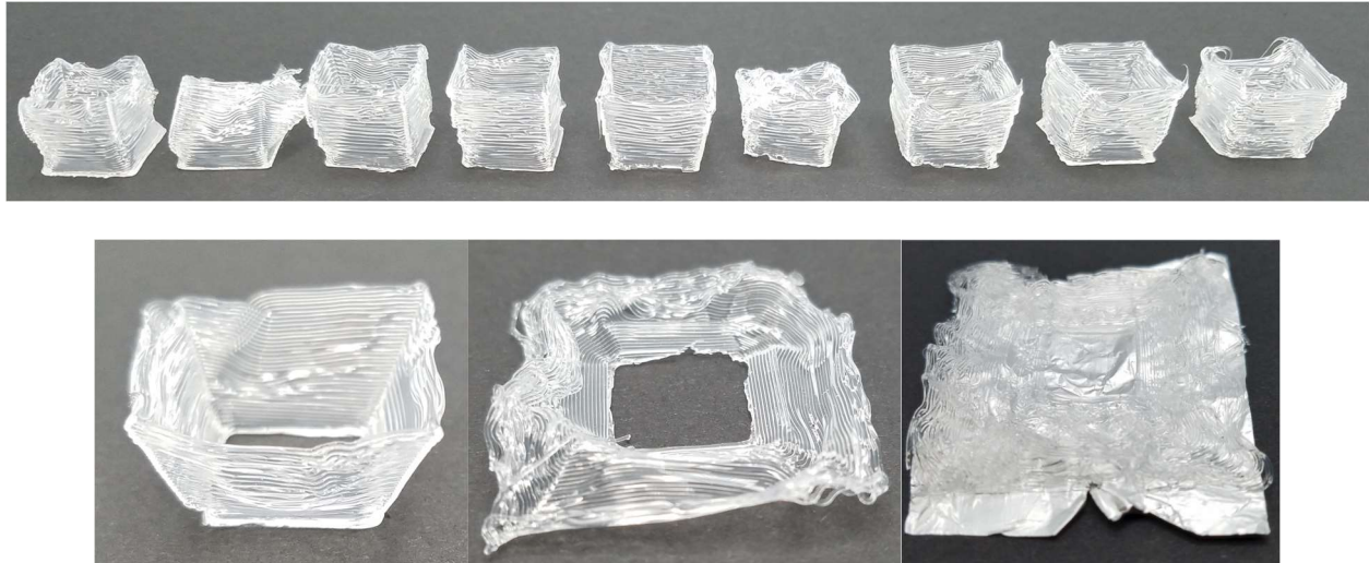
Figure 14: 1-9 Degree Overhang Tests (top row), 10-, 15-, and 20-Degree Overhang Tests (bottom row)
