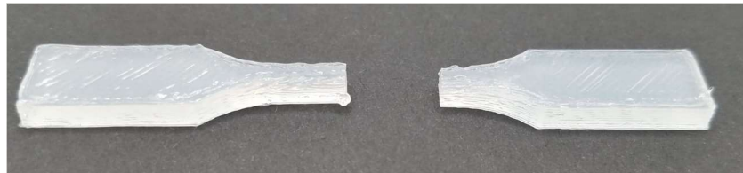
Figure 13: Tensile Beam After Testing
