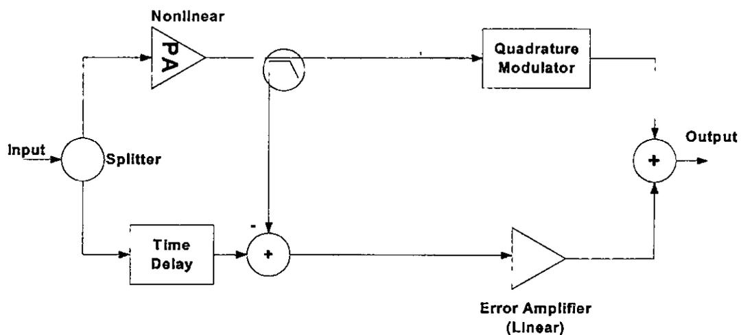
Figure 2.12 Block diagram of feed forward technique
