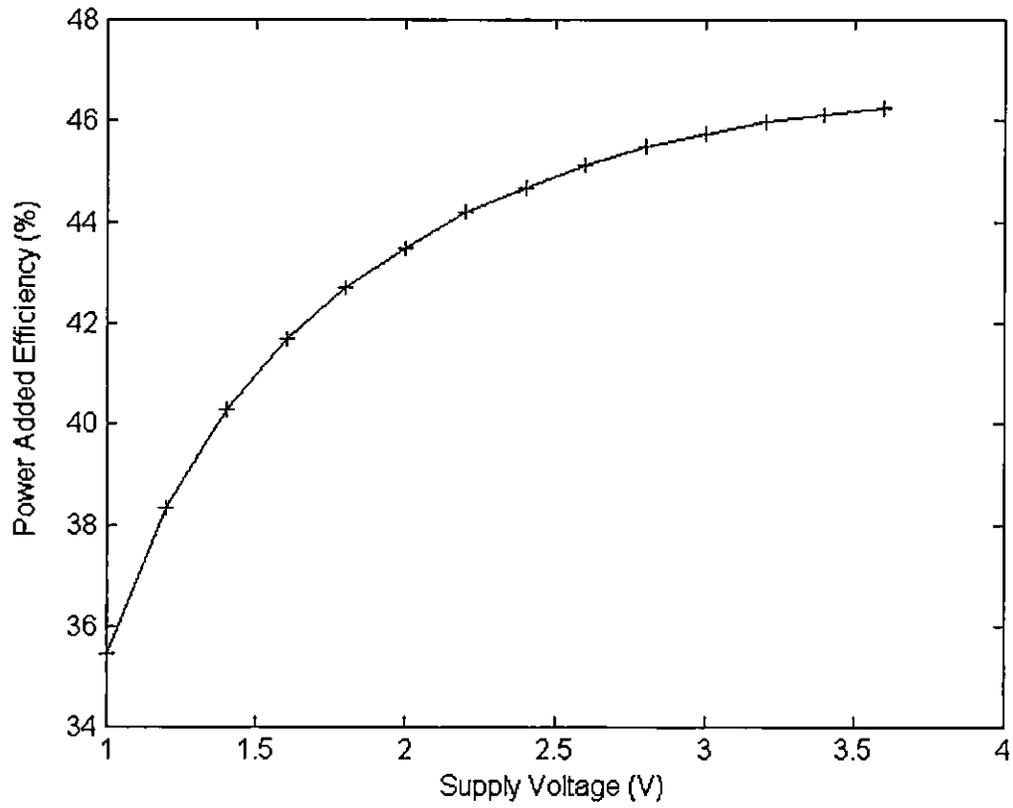
Figure 4.12 Simulated power added efficiency versus supply voltage
