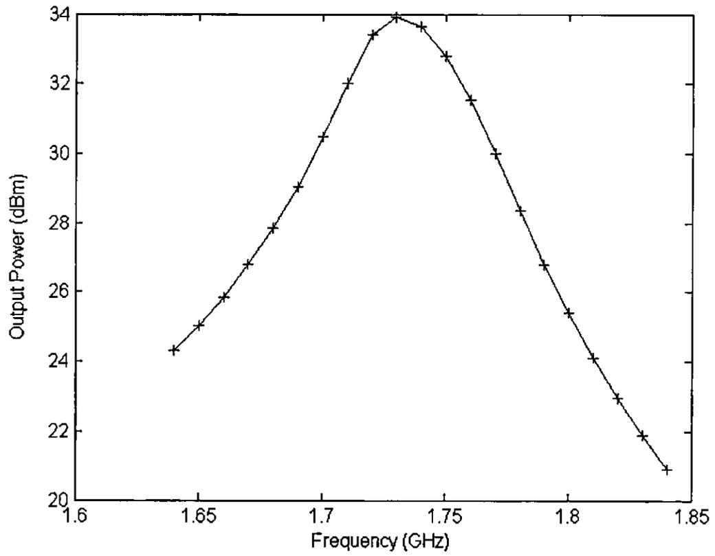
Figure 4.9 Simulated output power versus frequency
