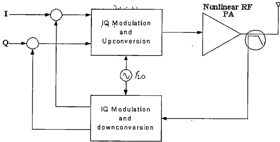
Figure 2.10 A block diagram of cartesian feedback linearization technique
