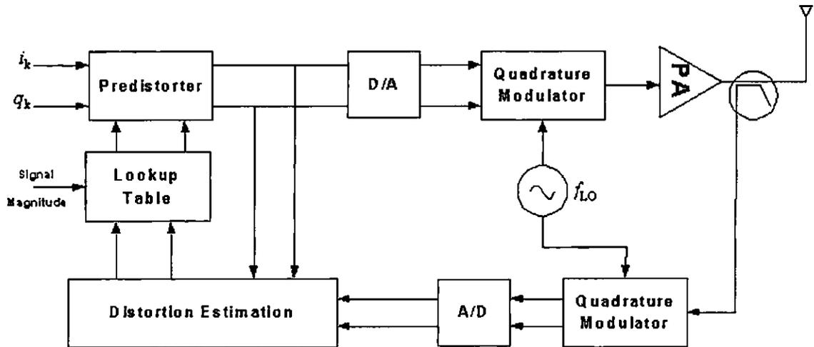
Figure 2.11 Block diagram of pre-distortion technique
