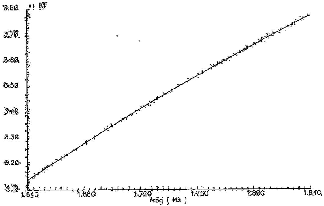
Figure 4.14 Stability factor (K) versus frequency
