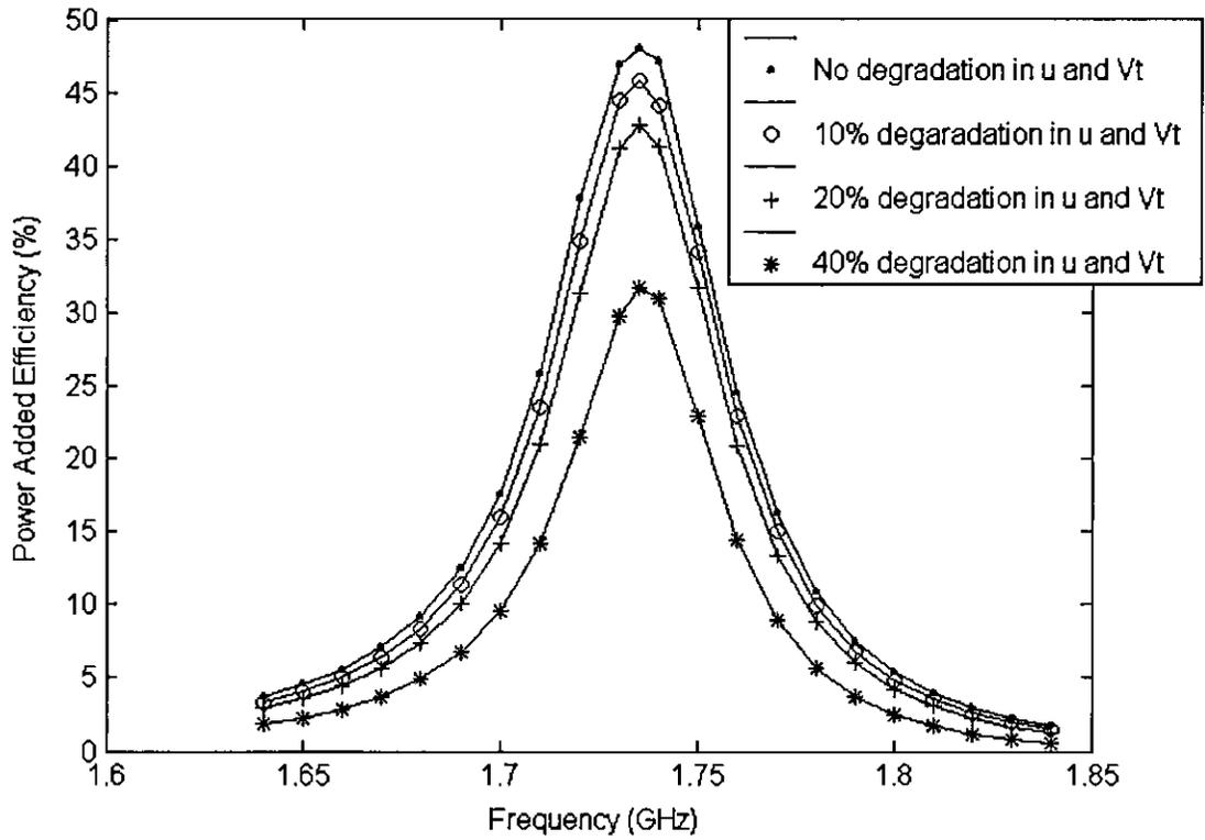
Figure 5.3 Power Added Efficiency degradation due to threshold voltage and mobility degradation
