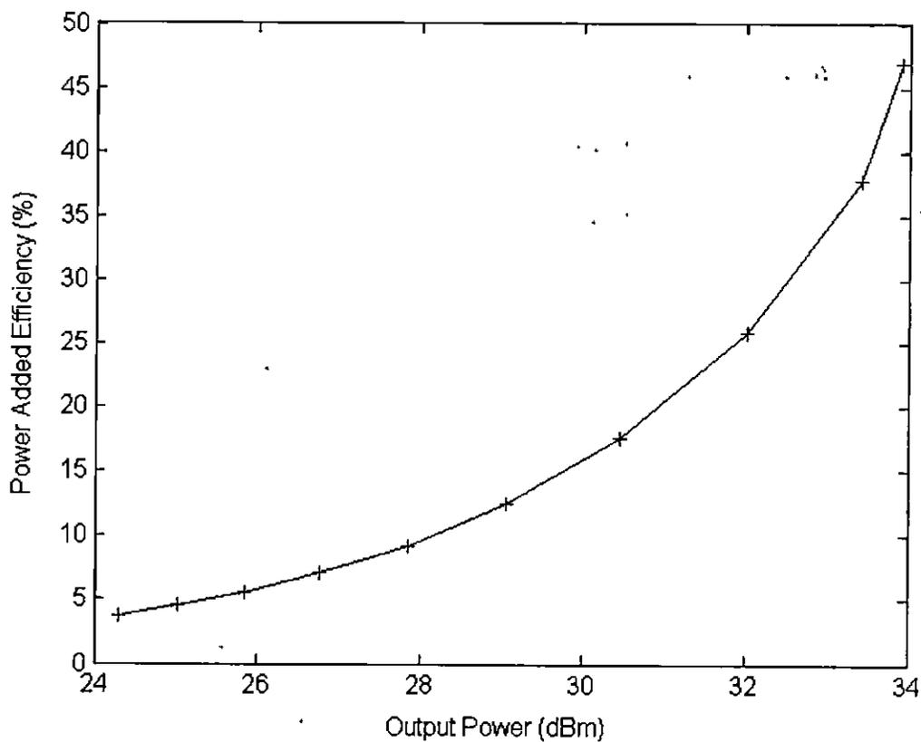
Figure 4.15 A plot of power added efficiency versus output Power
