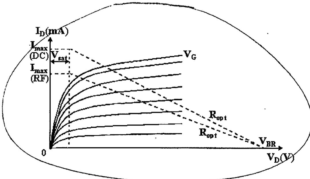
Figure 4.4 Optimum loading using load line approach
