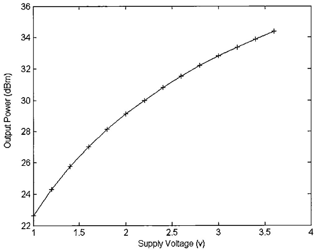
Figure 4.11 Simulated output power versus supply voltage
