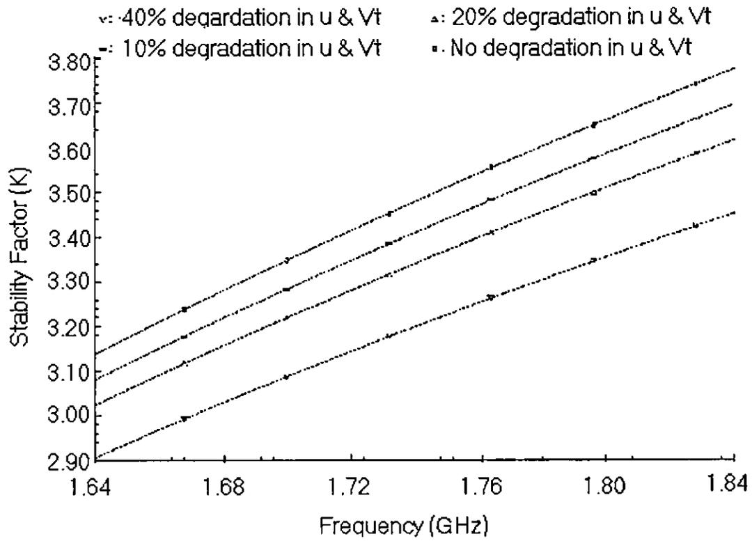
Figure 5.4 Stability factor (K) degradation due to threshold voltage and mobility degradation
