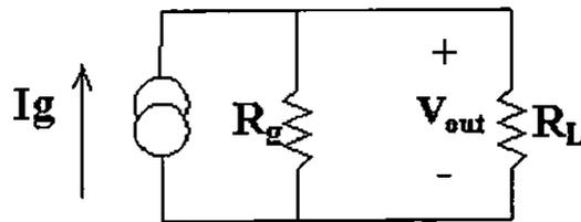
Figure 4.2 Schematic showing generator along with the load
