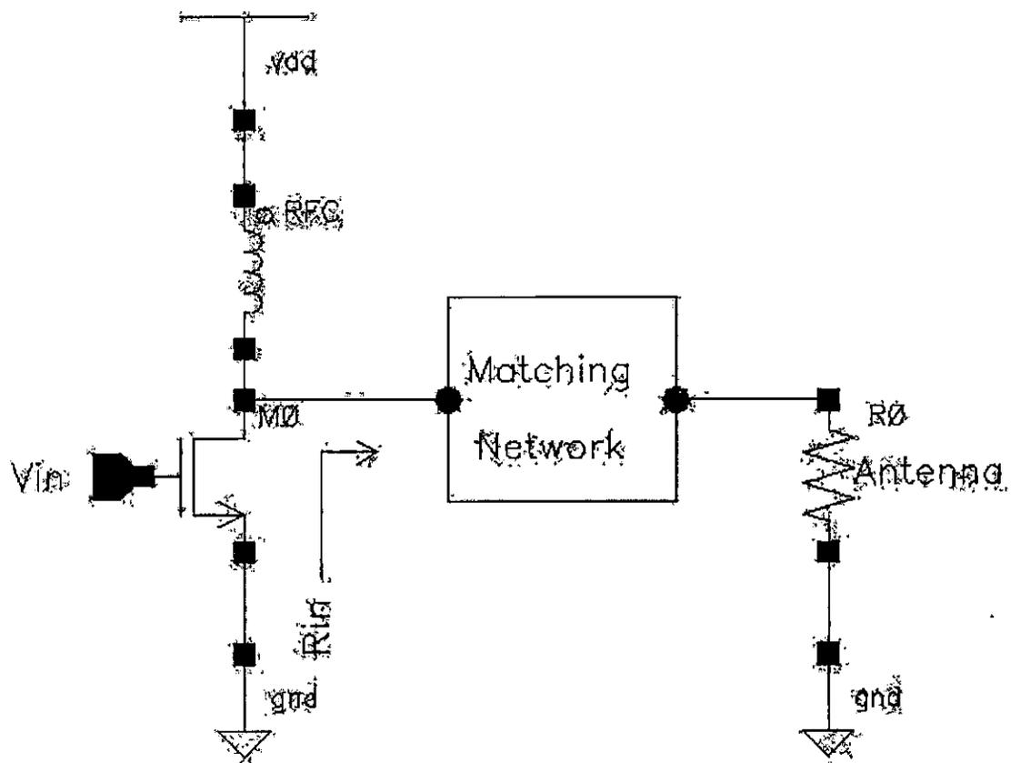
Figure 2.1 General circuit topology suitable for class A, AB, B, and C PAs.
