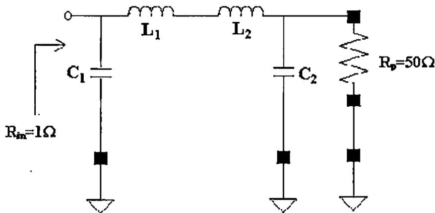
Figure 4.6  $\pi$ -matching network used in output matching network.
