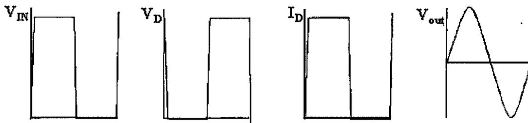
Figure 2.7 Class E waveforms
