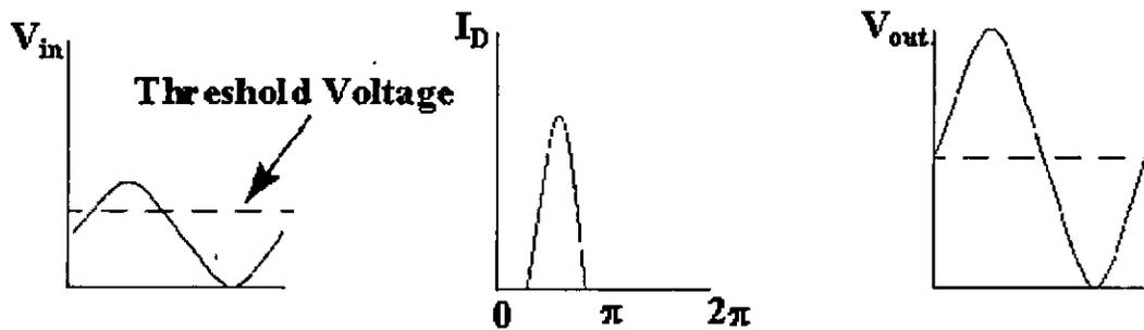
Figure 2.5 Input and output waveforms for class C PA
