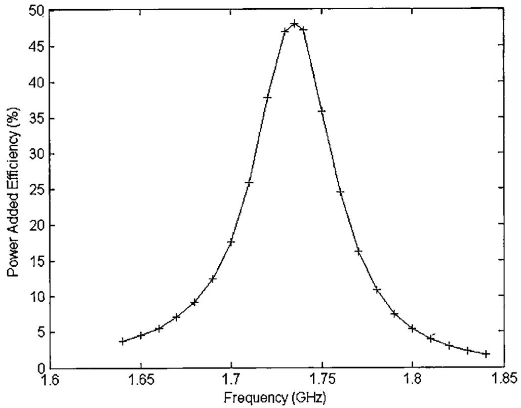
Figure 4.10 Simulated power added efficiency versus frequency
