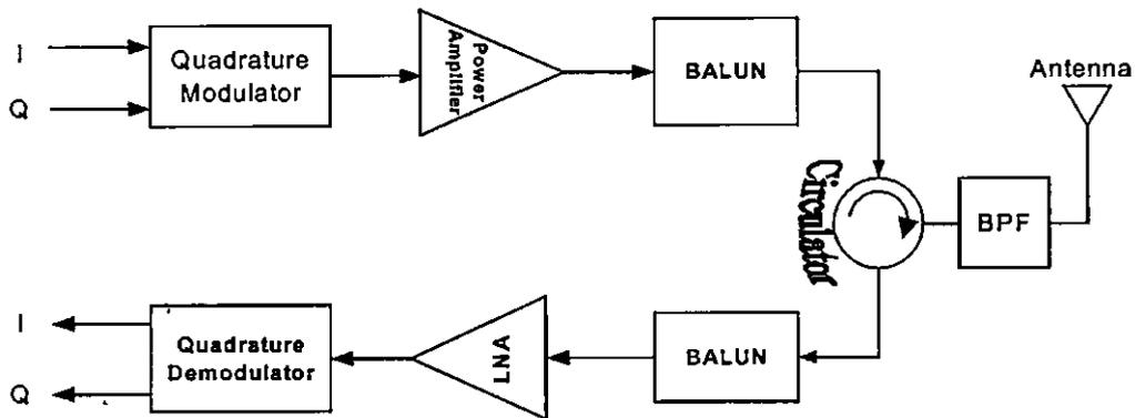
Figure 1.1 The structure of RF system.
