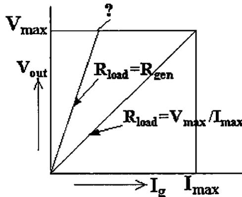
Figure 4.3 Output voltage versus current for a conjugate and load line match.
