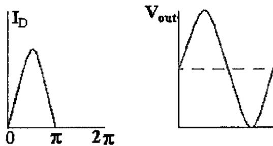
Figure 2.3 Class B waveforms
