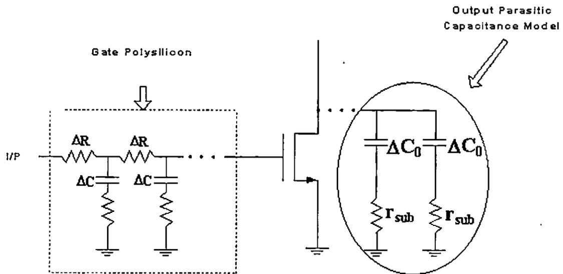
Figure 4.1 Input impedance and output junction capacitance model of device.
