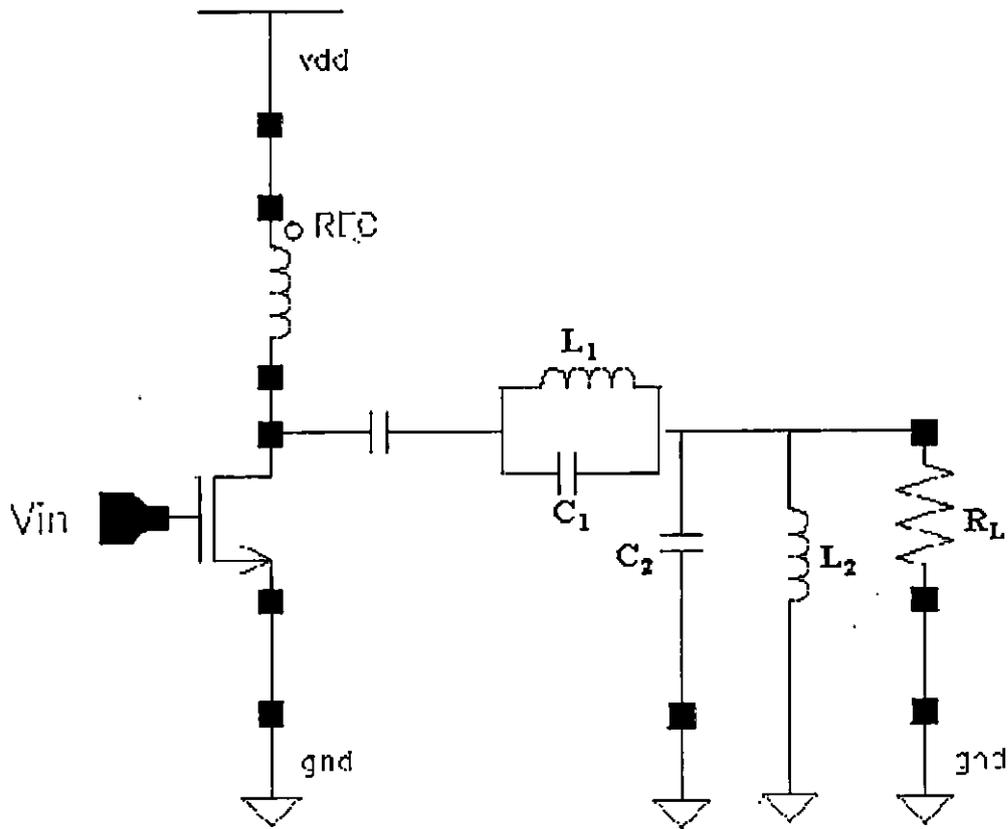
Figure 2.8 A typical class F stage circuit diagram
