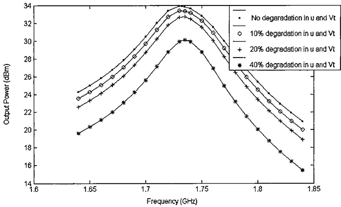
Figure 5.2 Output power degradation due to threshold voltage and mobility degradation
