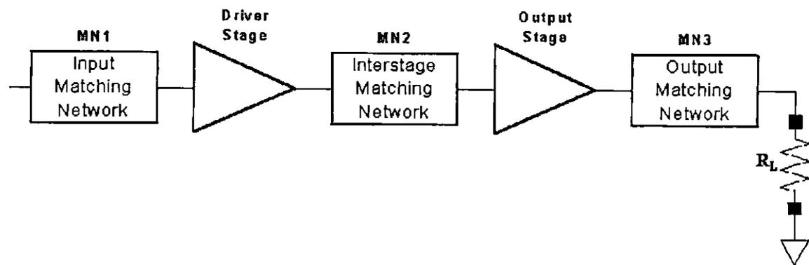
Figure 3.1 Multi-stage power amplifier circuit
