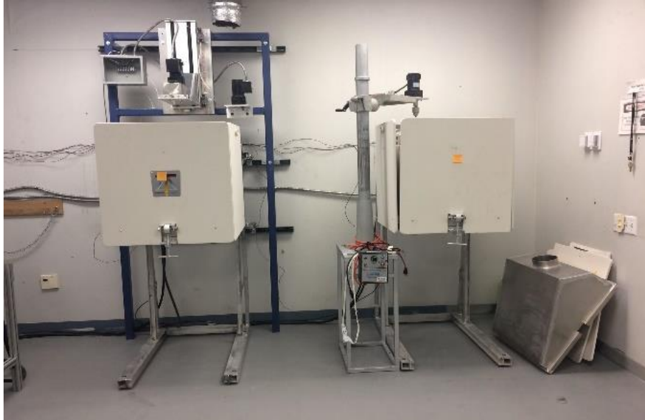
Figure 1-2 High-temperature glass melting furnaces installed in the glass laboratory at CREOL
