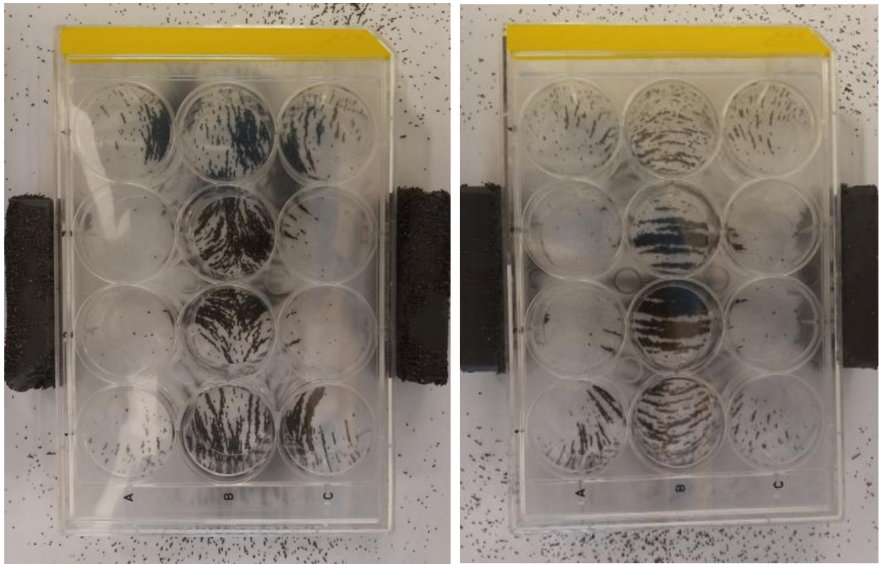
Figure 24: Visualization of magnetic field lines relative to 12 well dish positions. Left) Repulsive. Right) Attractive
