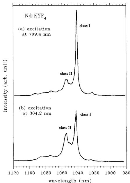
FIG. 1. Room-temperature emission spectra of Nd<sup>3+</sup>:KYF<sub>4</sub> in the 1  $\mu$ m region using excitation wavelengths of (a) 799.4 nm and (b) 804.2 nm.
