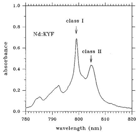
FIG. 2. Room-temperature absorption spectrum of  $\text{Nd}^{3+}:\text{KYF}_4$  in the 800 nm region. Arrows indicate the excitation wavelengths used in obtaining the emission spectra shown in Fig. 1.
