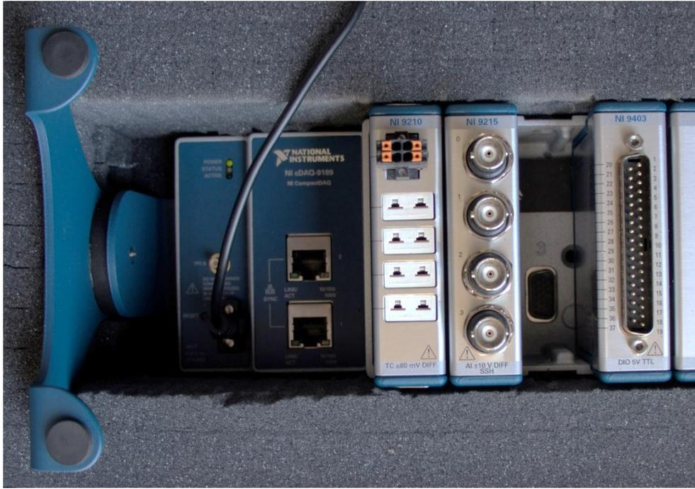
Figure 8. National Instruments data acquisition unit.
