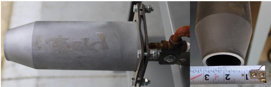
*Figure 4. Ceramic burner used in testing.*
