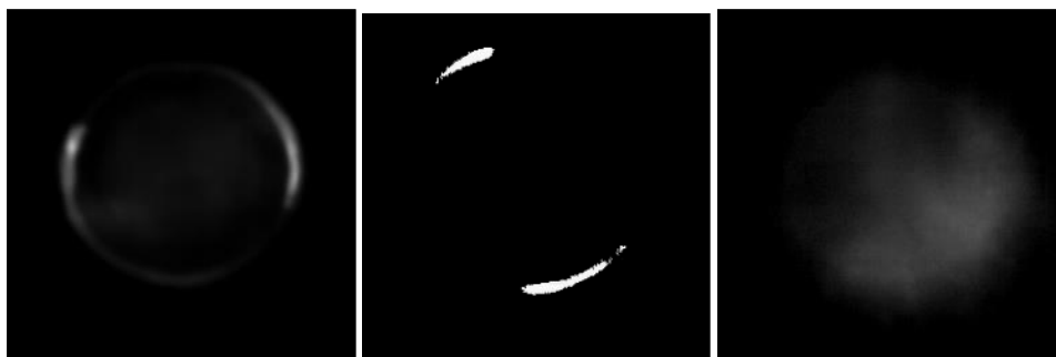
Figure 7: Back-end imaging of H 2 -Air detonating case (left), H 2 +Carbon Black-Air detonating case (mid), and H 2 +Peanut Flour-Air deflagrating case (right).
