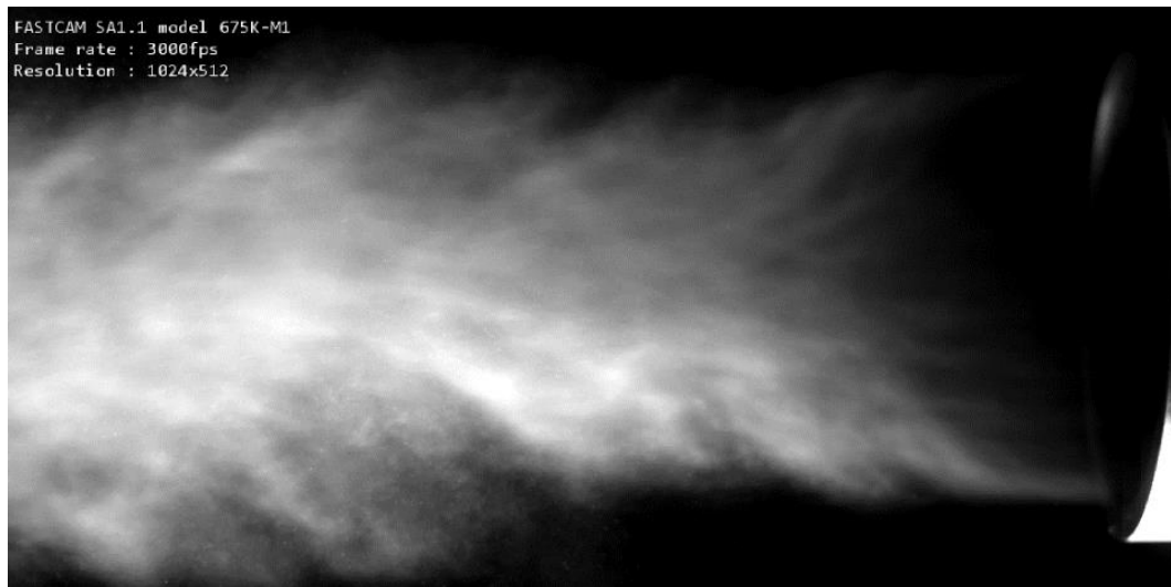
Figure 4: Particle seeding calibration using the Mie scattering technique.
