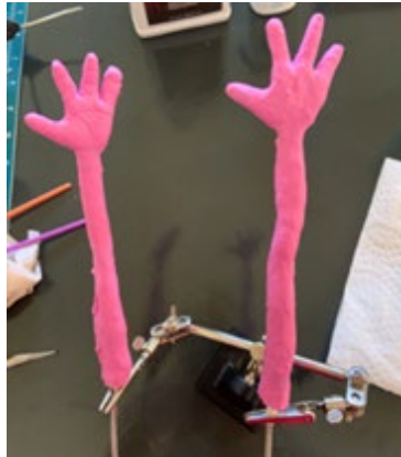
Figure 5: Silicone Hands Cast with Air Bubbles
