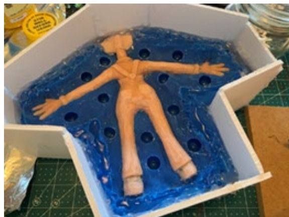
Figure 3: Mold Star 30 Layered On Armature
