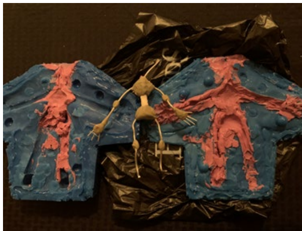
Figure 4: Failed Dragon Skin Mold Star 10
