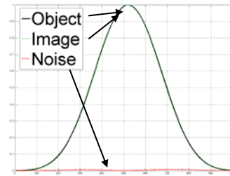
(s) The difference between both normalized autocorrelation of the object and image source cross-sections.
