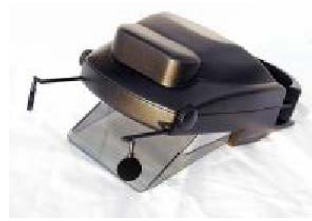
Figure 13: Head-mounted projection display
