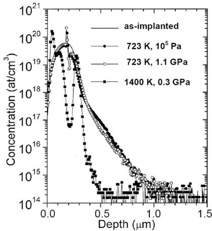
Fig. 1. Depth profiles of vanadium in Cz-Si:V ( $D = 1 \times 10^{15} \text{ cm}^{-2}$ ), as implanted and processed for 10 h at 723 K under  $10^5 \text{ Pa}$  and 1.1 GPa and for 5 h at 1400 K under 0.3 GPa.
