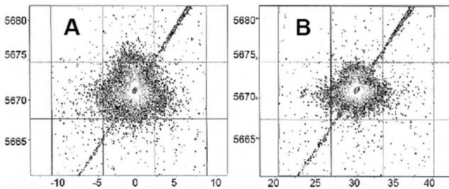
Fig. 6. XRRSMs of Cz-Si:V ( $D = 5 \times 10^{15} \text{ cm}^{-2}$ ), processed for 5 h at 1270 K under  $10^5 \text{ Pa}$  (A) and 1.12 GPa (B). Axis is given in  $\lambda/2d$  units ( $\lambda$  — wavelength,  $d$  — interplanar distance).
