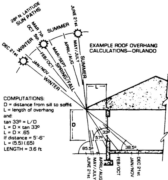
The Florida Solar Energy Center has compiled climatic data for various Florida locations and determined multiplication factors which appear optimum for the state's various latitudes. These functions, when multiplied by the distance from the window sill to the soffit, will provide adequate overhangs to protect against solar heat gain during the cooling season.
