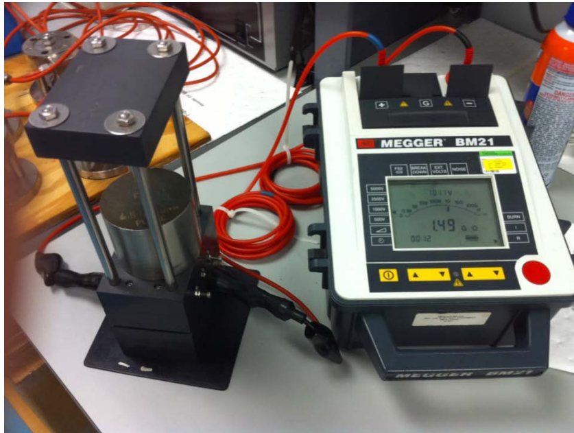
Figure 20: Equipment Setup for Insulation Resistance Measurement
