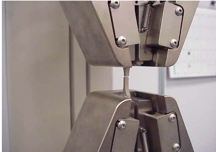
Figure 22: Specimen under tensile strength test
