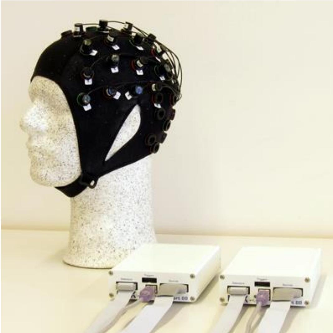
**Figure 2: NIRSport control systems and active-detection sensor cap**
