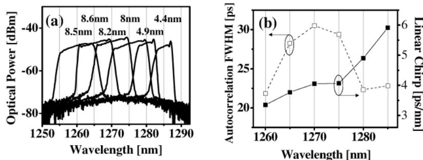
Fig. 2. (a) Optical spectra and (b) autocorrelation FWHM and linear chirp with respect to five different lasing spectral points.
