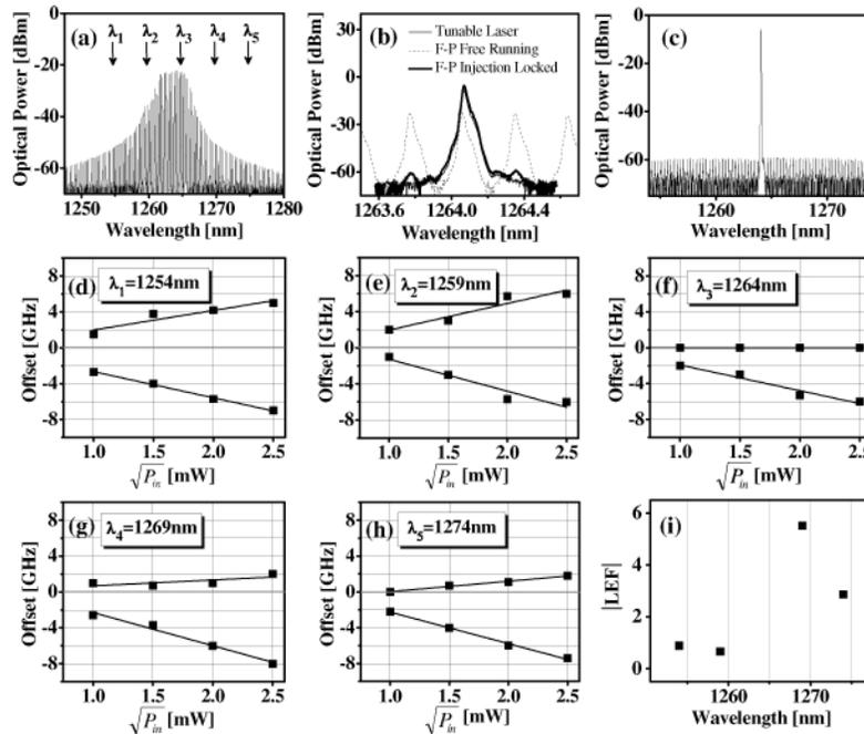
Fig. 1. (a) Optical spectrum of a free running QD F-P laser biased at 45 mA (5 arrows indicate measurement points for LEF), (b) Optical spectra of QD F-P laser before and after injection locking, (c) wide span optical spectrum of injection locked QD F-P laser, (d) ~ (h) injection locking bandwidth with different lasing spectral points, and (i) LEF as function of wavelength.
