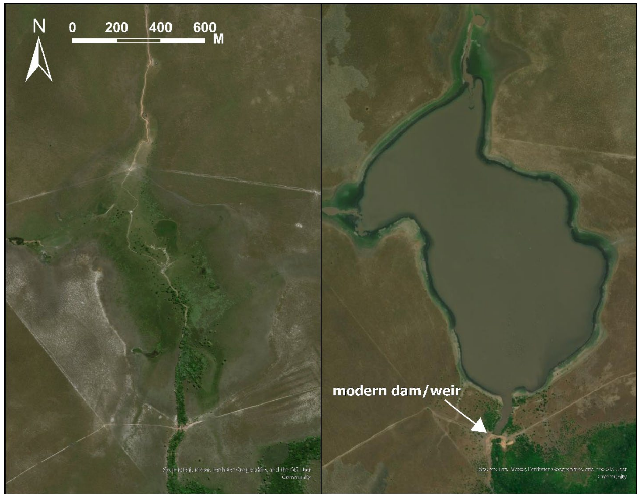
Figure 7. The location of the artificial lake north of Santa Ana del Yacuma, in 2013 (left) and in 2017 (right) after the strategic construction of a low dam or weir within the channel of a seasonal stream. This demonstrates how the flow and accumulation of water can be impacted by relatively small, linear features. Imagery from 2014-2016 was not available for preview in the World Imagery Wayback archive.
