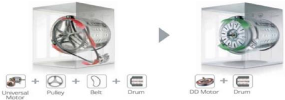
Figure 12: Belt driven motor vs direct drive motor in washing machine systems [16]
