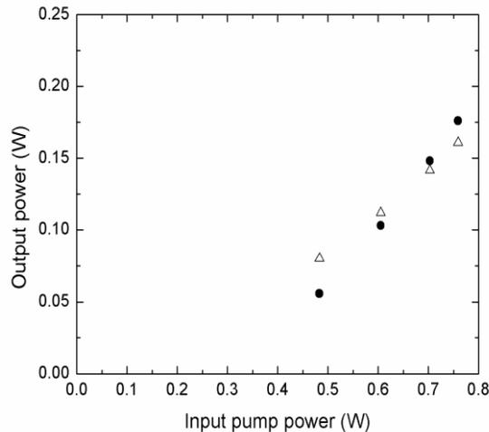
Fig. 2. The calculated output laser power (open triangles) versus the input pump power before entering the Cs cell, together with the experimental results (solid circles) presented in [1]. The output coupler reflectivity used in the calculation and in the experiment is 0.5.
