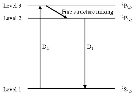
Fig. 1. Schematic energy level diagram for alkali metal vapors.
