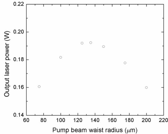
Fig. 4. The calculated output laser power versus the pump beam waist radius at  $1/e^2$  of the axial intensity.
