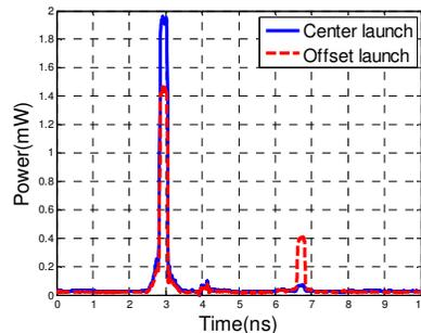
Fig. 5. Impulse response of a FMF at 1550nm.
