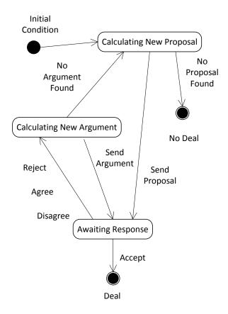
Figure 6.2: Radio Node Negotiation State Diagram.
