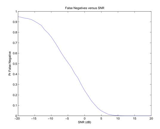
Figure 3.7: Probability of False Negatives Versus SNR
