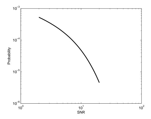
Figure 3.2: Probability of false positive versus signal to noise ratio
