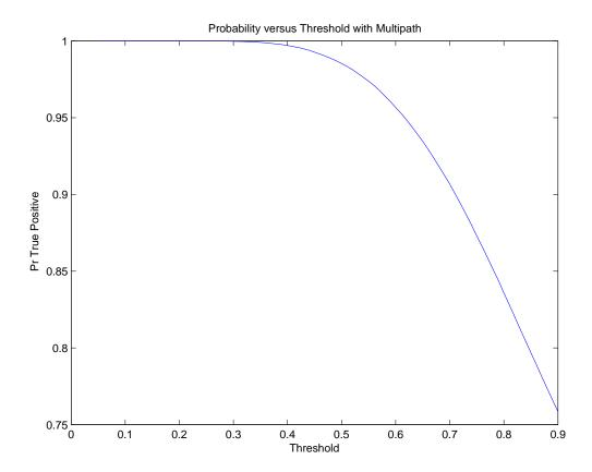
Figure 3.9: Probability of Probe Signal Detection Versus Threshold with Multipath
