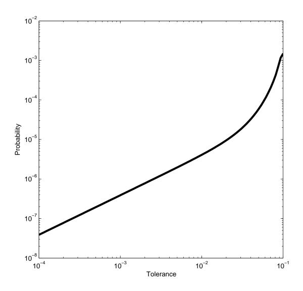
Figure 3.3: Probability of false positive versus tolerance window
