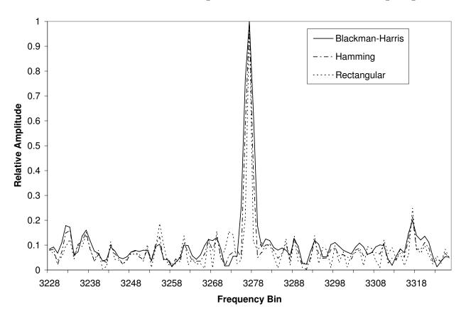
Figure 4.5: Three Window Functions
