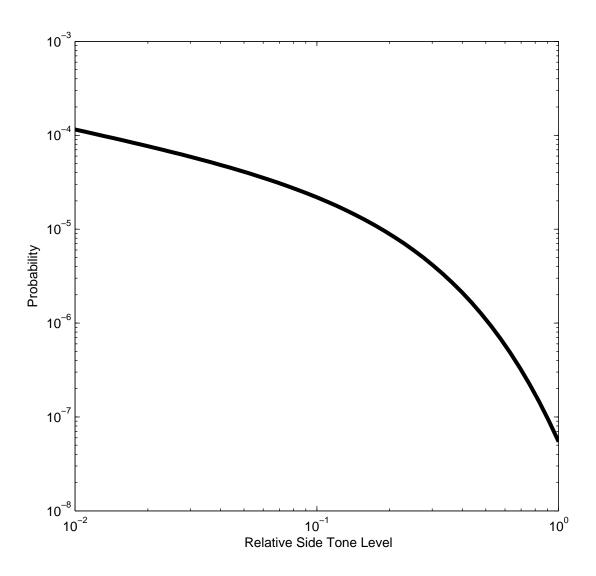
Figure 3.1: Probability of false positive versus relative amplitude of tones
