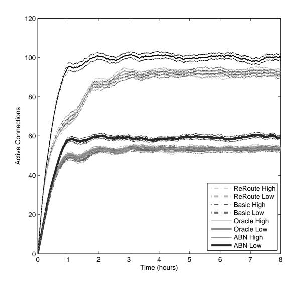
Figure 8.6: Total Active Connections With High Request Rate Sparsely Connected Network
