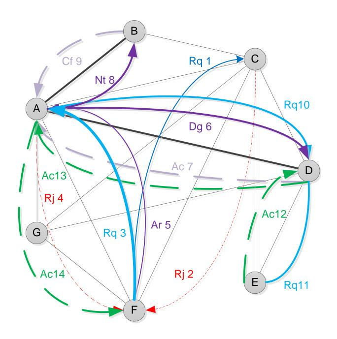
Figure 8.3: Message exchange including downgrade and notify messages
