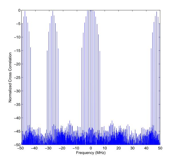
Figure 4.3: Cross-Correlation for 5 Sent Channels at 0 dB SNR
