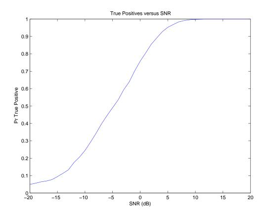
Figure 3.5: Probability of Probe Signal Detection Versus SNR
