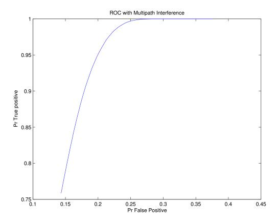
Figure 3.8: Receiver Operating Characteristic for Multi-Tone probe signal with varying threshold
