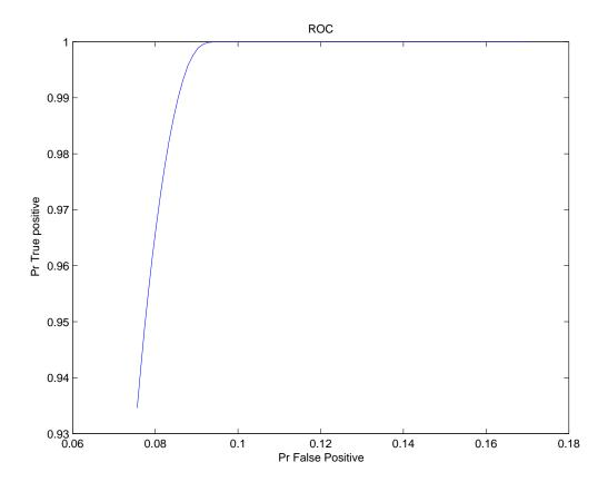
Figure 3.6: Receiver Operating Characteristic for Multi-Tone Probe Signal with Varying Threshold
