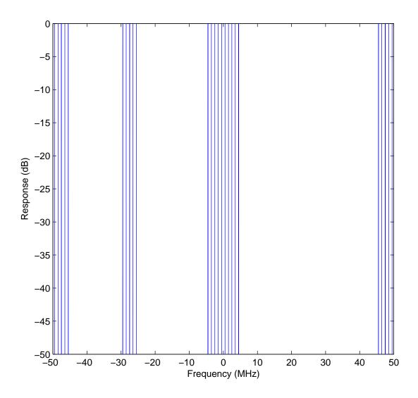
Figure 4.1: Spectrum for 5 Sent Channels as Transmitted
