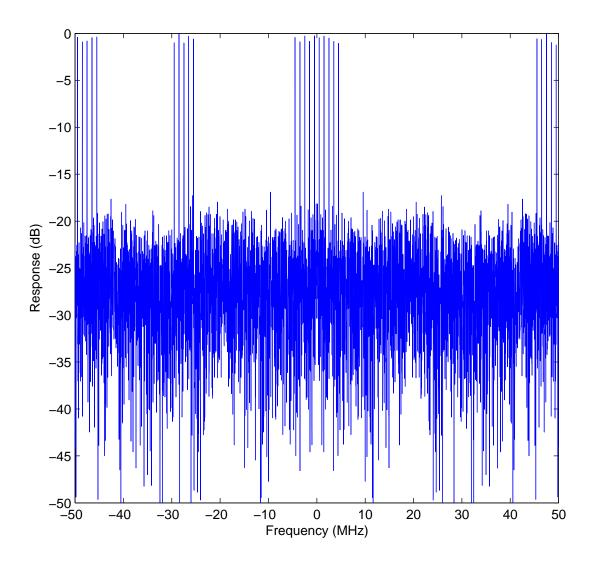
Figure 4.2: Spectrum for 5 Sent Channels Received at 0 dB SNR
