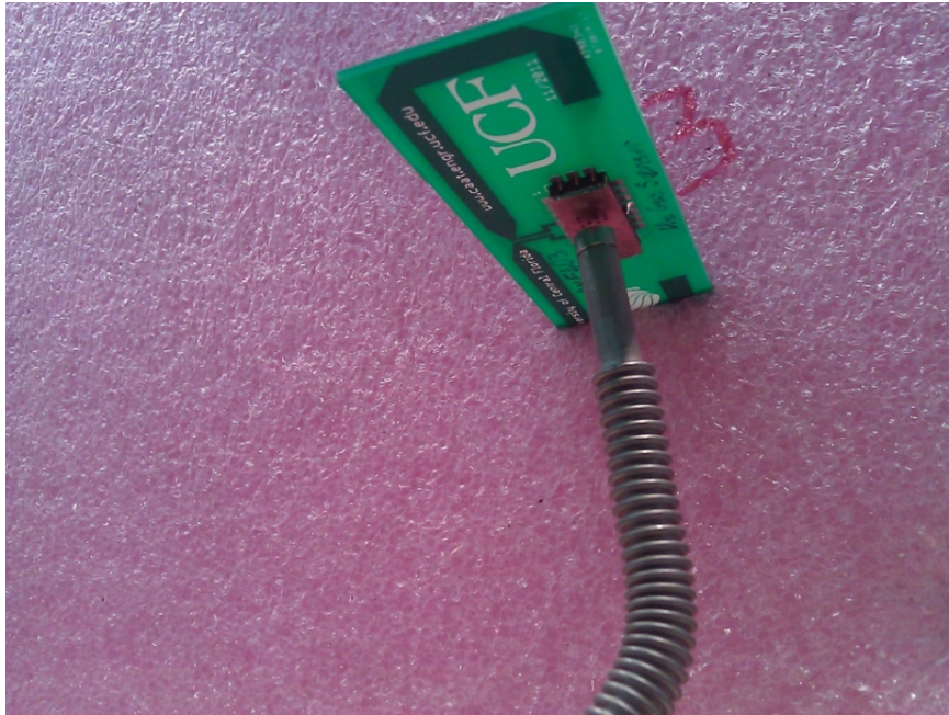
Figure 7-11. A picture of the gas flow tube filling gas precisely onto the SnO 2 film.
