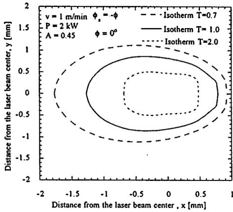
FIG. 5. Top surface ( $z=0$ ) isotherms for a laser beam ( $TEM_{mn}$ ,  $m=0,1$ , and  $n=0,1$ ) of spot size  $2l_s=1.7$  mm and  $2w_s=1.2$  mm, moving in positive  $x$  direction with a speed  $v$  and scanning angle  $\phi_s=0$ .
