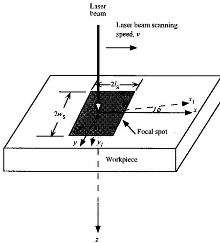
FIG. 1. The laser spot in relation to the rotated  $(x_1, y_1)$  and unrotated  $(x, y)$  coordinates, scanning in the positive  $x$  direction with a constant speed  $v$ . For further detail see Fig. 2.
