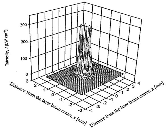
FIG. 3. Intensity distribution ( $P=2$  kW) at the focal spot for a laser beam (TEM<sub>*m*n</sub>,  $m=0,1$ , and  $n=0,1$ ) of spot size  $2l_s=1.7$  mm and  $2w_s=1.2$  mm, moving in positive  $x$  direction with a speed  $v=1$  m/min. Scanning angle  $\phi_s=0$ .
