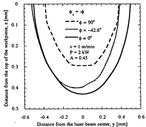
FIG. 11. Melt pool shapes at the slice  $x=-1.1$  mm for the laser beam ( $TEM_{mn}$ ,  $m=0,1$ , and  $n=0,1$ ) of spot size  $2l_s=1.7$  mm and  $2w_s=1.2$  mm for different scanning angles,  $\phi_s = -\phi$ .
