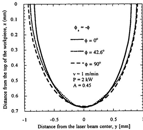
FIG. 9. Melt pool shapes at the slice  $x=0$  mm for the laser beam ( $TEM_{mn}$ ,  $m=0,1$ , and  $n=0,1$ ) of spot size  $2l_s=1.7$  mm and  $2w_s=1.2$  mm for different scanning angles,  $\phi_s = -\phi$ .
