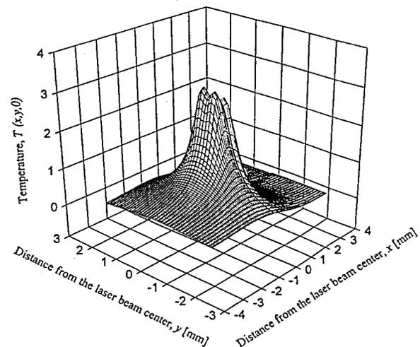
FIG. 4. Temperature distribution ( $P=2$  kW,  $A=0.45$ ) at the top of workpiece ( $z=0$ ), for a laser beam (TEM<sub>*m*n</sub>,  $m=0,1$ , and  $n=0,1$ ) of spot size  $2l_s=1.7$  mm and  $2w_s=1.2$  mm, moving in positive  $x$  direction with a speed  $v=1$  m/min. Scanning angle  $\phi_s=0$ .
