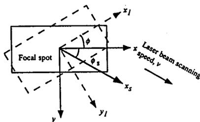
FIG. 2. The focal spot is rotated through an angle  $\phi$ , and is scanned along the positive  $x$  direction with a constant speed  $v$ . It has the same heating effect as keeping the focal spot unrotated and scanning it at an angle  $\phi_s$ , along  $x_s$  direction with a constant speed  $v$ , such that  $\phi_s = -\phi$ .
