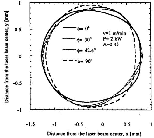
FIG. 7. Melt pool shapes ( $z=0$ ) for the laser beam ( $TEM_{mn}$ ,  $m=0,1$ , and  $n=0,1$ ) of spot size  $2l_s=1.7$  mm and  $2w_s=1.2$  mm for different scanning angles,  $\phi_s=-\phi$ .
