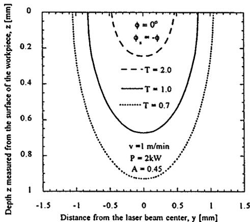
FIG. 6. Isotherms in the  $y-z$  plane at  $x=0$ , for a laser beam ( $TEM_{mn}$ ,  $m=0,1$ , and  $n=0,1$ ) of spot size  $2l_s=1.7$  mm and  $2w_s=1.2$  mm. Scanning angle  $\phi_s=0$ .
