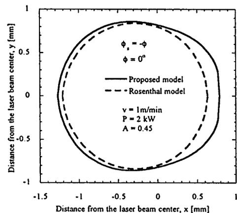
FIG. 12. Melt pool comparison ( $z=0$ ) between proposed model and Rosenthal model. The laser beam ( $TEM_{mn}$ ,  $m=0,1$ , and  $n=0,1$ ) of spot size  $2l_s=1.7$  mm and  $2w_s=1.2$  mm is used for proposed model.
