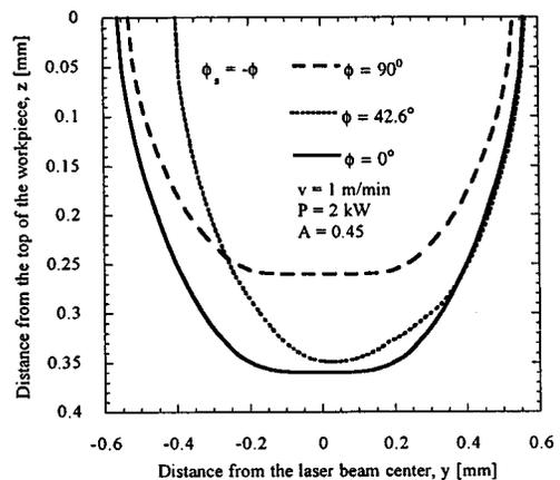
FIG. 8. Melt pool shapes at the slice  $x=0.6$  mm for the laser beam ( $TEM_{mn}$ ,  $m=0,1$ , and  $n=0,1$ ) of spot size  $2l_s=1.7$  mm and  $2w_s=1.2$  mm for different scanning angles,  $\phi_s=-\phi$ .
