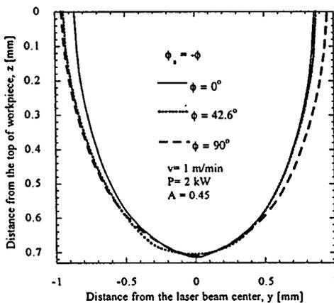
FIG. 10. Melt pool shapes at the slice  $x=-0.345$  mm for the laser beam ( $TEM_{mn}$ ,  $m=0,1$ , and  $n=0,1$ ) of spot size  $2l_s=1.7$  mm and  $2w_s=1.2$  mm for different scanning angles,  $\phi_s = -\phi$ .
