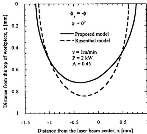
FIG. 13. Melt pool comparison ( $y=0$ ) between proposed model and Rosenthal model. The laser beam ( $TEM_{mn}$ ,  $m=0,1$ , and  $n=0,1$ ) of spot size  $2l_s=1.7$  mm and  $2w_s=1.2$  mm is used for proposed model.
