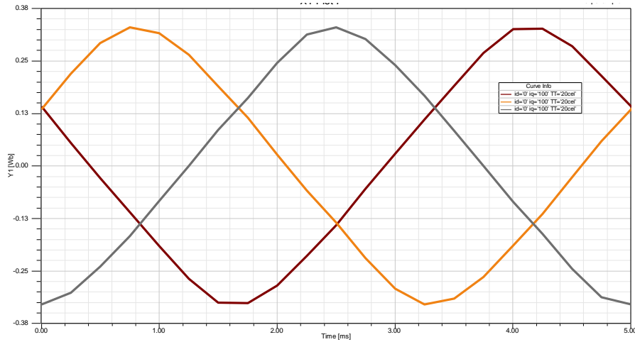
Figure 5.7: 3 phase flux linkages in abc reference frame for i_d = 0 A, i_q = 100 A, temperature = 20 °C
