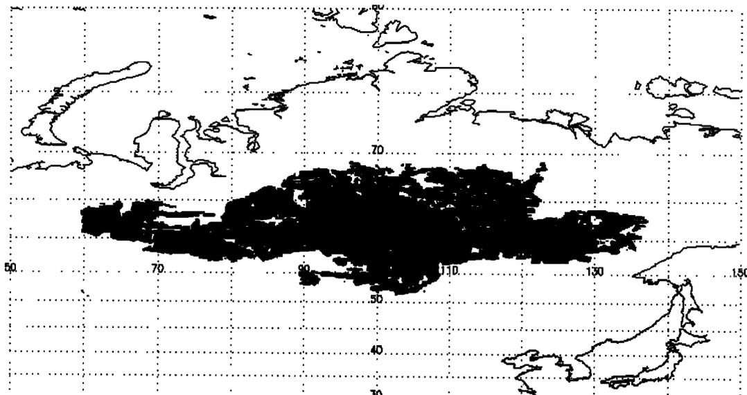
Figure 3. Siberian mask used for data editing. Black pixels are within  $\pm 0.5$  dB of the mean  $\sigma^0$ .
