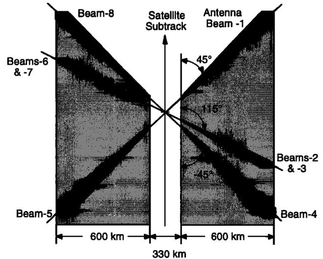
Figure 1. NASA scatterometer (NSCAT) antenna illumination patterns.
