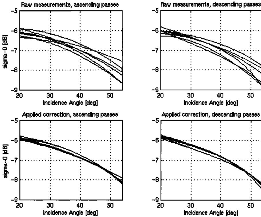
Figure 13. Effects of corrections on beam response for Amazon, November 1996.
