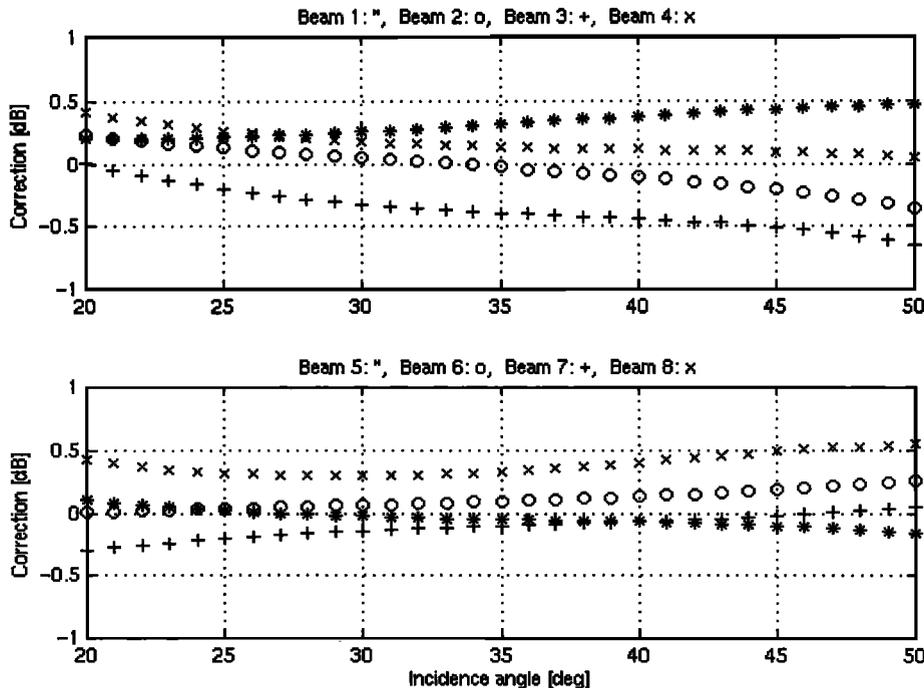
Figure 9. Beam corrections based on Amazon November 1996 data.
