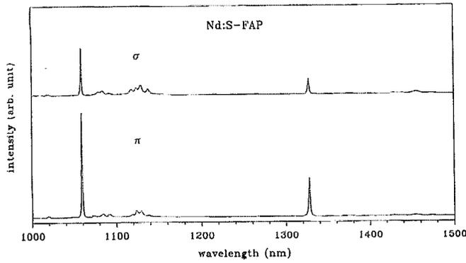
FIG. 2. Room temperature polarized emission spectra of Nd<sup>3+</sup>:S-FAP in the 1.06- and 1.33- $\mu\text{m}$  regions obtained by cw excitation at 805.4 nm.
