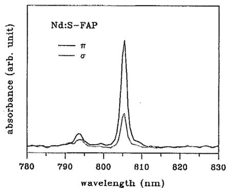
FIG. 1. Room temperature polarized absorption spectra of Nd<sup>3+</sup>:S-FAP in the 800-nm region.
