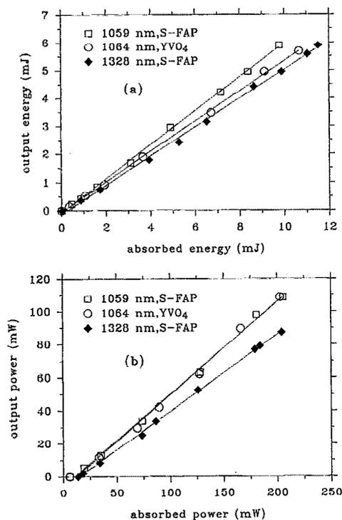
FIG. 3. The input/output characteristics of  $\text{Nd}^{3+}$ :S-FAP and  $\text{Nd}^{3+}$ : $\text{YVO}_4$  for (a) pulsed and (b) cw operation.
