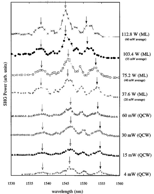
FIG. 4. Wavelength scan in the LiNbO<sub>3</sub> QPM waveguide at different peak powers in the vicinity of the interaction  $TM_{00}(\omega) \rightarrow TM_{02}(2\omega) + TM_{40}(2\omega) + TM_{21}(2\omega)$ . These curves were normalized to the solid arrow points in Fig. 3. Point (open and solid) arrows track the position of the peak conversion to the  $TM_{21}(TM_{40}$  and  $TM_{02})$  mode.
