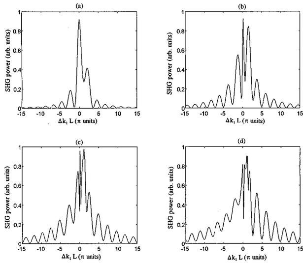
FIG. 1. SHG detuning curve for different normalized input powers. (a)  $I_0=0.25$ , (b)  $I_0=1.0$ , (c)  $I_0=2.25$ , and (d)  $I_0=4.0$ . In all cases  $\kappa_1L=4$ ,  $\kappa_2L=1.5$ , and  $\Delta k_0L=2\pi$ .
