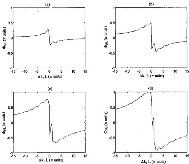
FIG. 2. Total nonlinear phase shift for (a)  $I_0=0.25$ , (b)  $I_0=1.0$ , (c)  $I_0=2.25$ , and (d)  $I_0=4.0$ . In all cases  $\kappa_1L=4$ ,  $\kappa_2L=1.5$ , and  $\Delta k_0L=2\pi$ .
