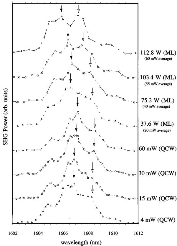
FIG. 3. Wavelength scan in the LiNbO<sub>3</sub> QPM waveguide at different peak powers in the vicinity of  $TM_{00}(\omega) \rightarrow TM_{01}(2\omega) + TM_{20}(2\omega)$ . Solid (open) arrows track the position of the peak conversion to the  $TM_{01}(TM_{20})$  mode. Conversion efficiencies on the solid arrows for these curves are (bottom to top): 0.005%, 0.069%, 0.33%, 0.63%, 17%, 21%, 23%, and 27%, respectively.
