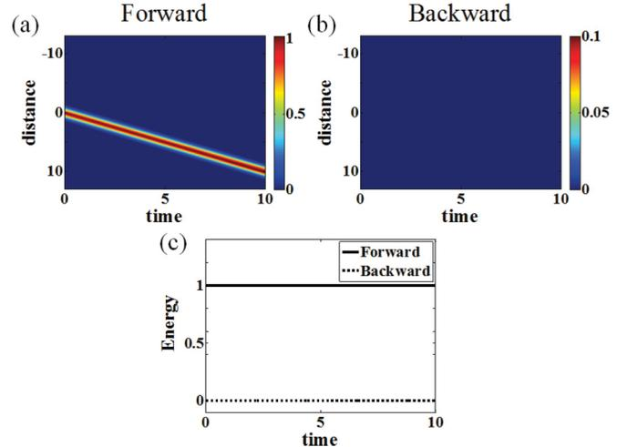
FIG. 4. (Color online) The same as Fig. 3 when the  $\mathcal{PT}$  grating is operated at the  $\mathcal{PT}$ -symmetry breaking threshold. (a),(b) Forward and backward components, respectively, and (c) the associated energy as a function of normalized time.
