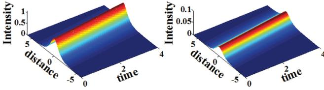
FIG. 2. (Color online) Propagation dynamics of a solitary wave solution in a  $\mathcal{PT}$ -symmetric Bragg structure; intensity evolution for both the forward (left) and backward waves (right) during propagation.
