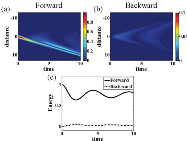
FIG. 3. (Color online) Propagation dynamics of a Gaussian wave packet when injected only in the forward direction when the  $\mathcal{PT}$  grating is operated below the  $\mathcal{PT}$ -symmetry breaking threshold. (a),(b) Forward and backward components, respectively, and (c) the associated energy as a function of normalized time.
