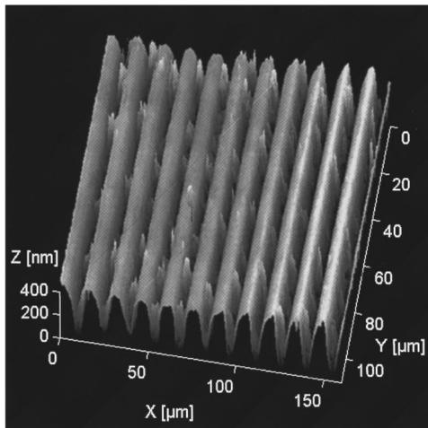
FIG. 2. Three-dimensional surface plot of the periodically poled sample with digital electrode on the multilayer stack surface. Maximum deformation amplitude is larger than 300 nm.
