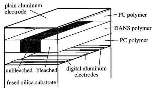
FIG. 1. Sample geometry with periodic electrode ( $\Lambda = 14 \mu\text{m}$ ) on the substrate.
