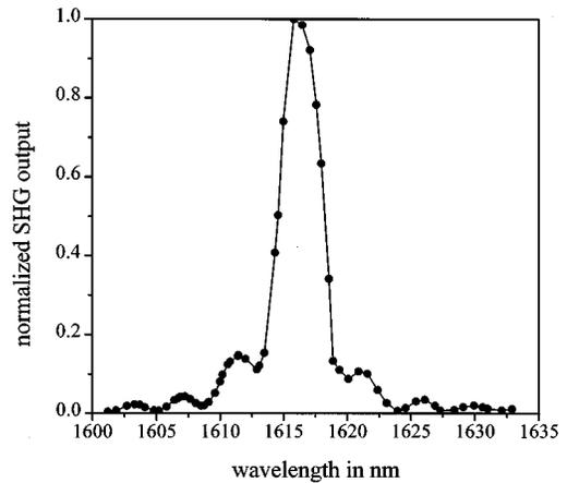
FIG. 3. Normalized second-harmonic output vs detuning. The acceptance bandwidth corresponds to a phase-matching length of 0.2 cm.
