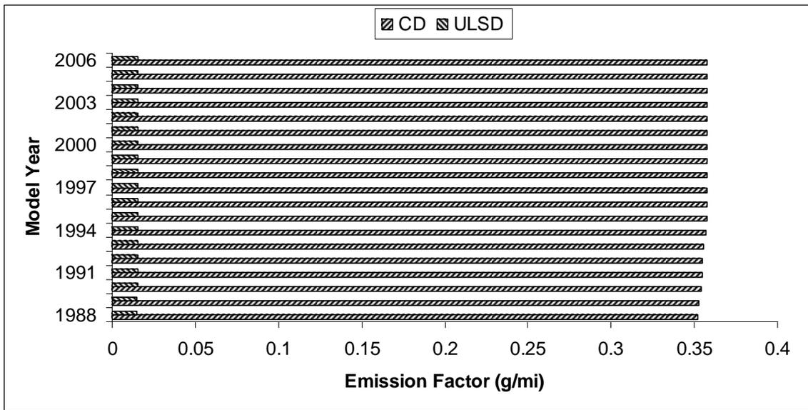
**Figure 2-11: The effects of CD and ULSD on SO<sub>2</sub> emissions**
