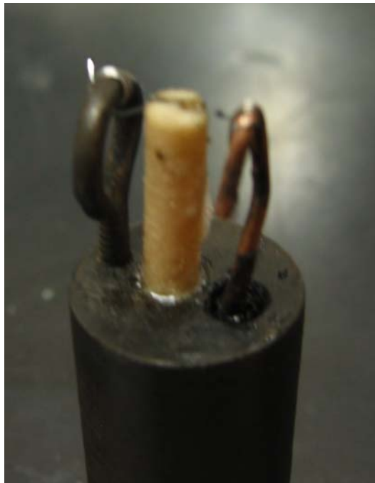
Figure 10: An AP / HTPB Ready to be Loaded Into the Strand Burner
