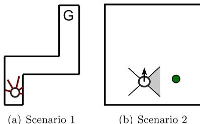
**Figure 6.** Dual task. In the dual task domain the agent has to exhibit either wall-following (a) or food-gathering behavior (b), depending on the type of sensory input it receives.
