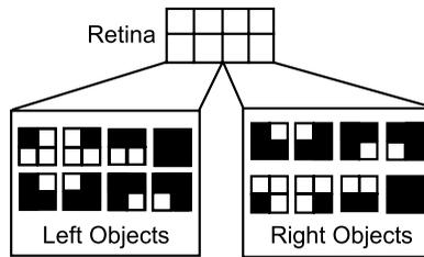
Figure 15. Retina problem. The artificial retina consists of  $4 \times 2$  pixels that constitute the inputs to the ANN. Eight out of 16 possible patterns are considered left objects. The same is true for the right four pixels, though the eight valid patterns are different. The picture is adapted from Kashtan and Alon [29].
