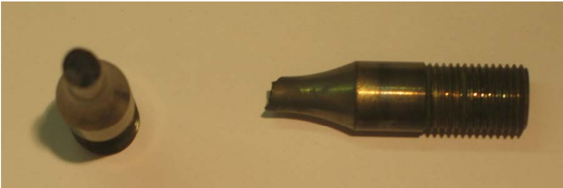
Figure A.22. Photograph of fractured specimen D912-8, 750°C test temp and 0.199 norm. strain range.
