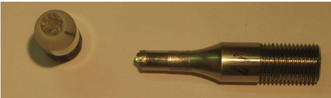
Figure A.13. Photograph of fractured specimen D912-17, 24°C test temp and 0.184 norm. strain range.
