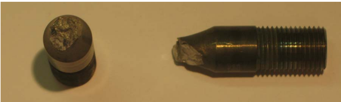
Figure A.20. Photograph of fractured specimen D912-6, 750°C test temp and 0.150 norm. strain range.
