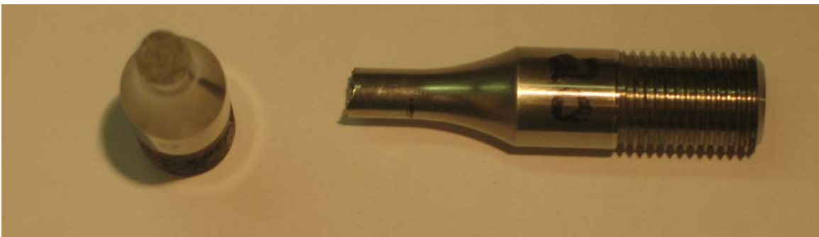
Figure A.14. Photograph of fractured specimen D912-20, 24°C test temp and 0.222 norm. strain range.
