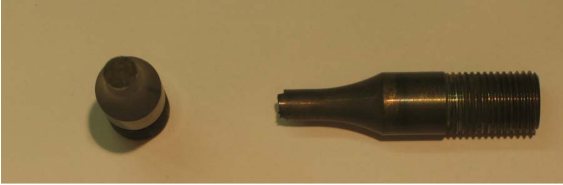
Figure A.21. Photograph of fractured specimen D912-14, 750°C test temp and 0.174 norm. strain range.
