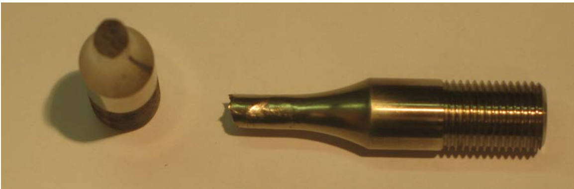
Figure A.17. Photograph of fractured specimen D912-33, 400°C test temp and 0.177 norm. strain range.
