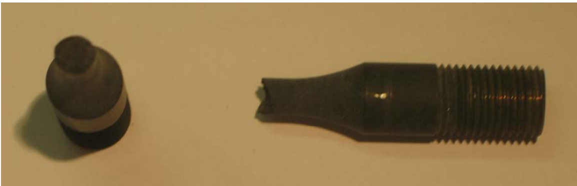
Figure A.23. Photograph of fractured specimen D912-16, 850°C test temp and 0.116 norm. strain range.
