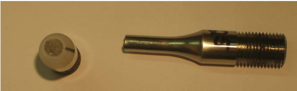
Figure A.16. Photograph of fractured specimen D912-25, 24°C test temp and 0.294 norm. strain range.
