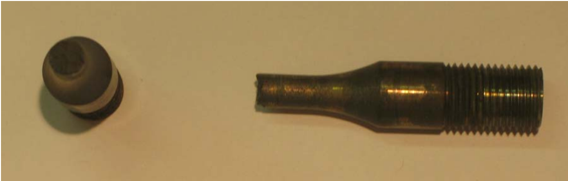
Figure A.25. Photograph of fractured specimen D912-11, 850°C test temp and 0.155 norm. strain range.
