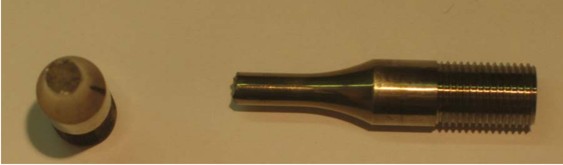
Figure A.18. Photograph of fractured specimen D912-1, 400°C test temp and 0.222 norm. strain range.
