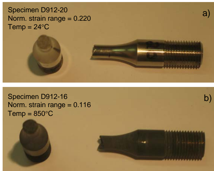
Figure 4.3. Photographs of failed specimens at 24°C and 850°C.
