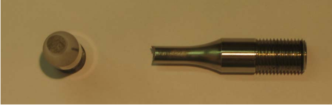
Figure A.15. Photograph of fractured specimen D912-19, 24°C test temp and 0.257 norm. strain range.
