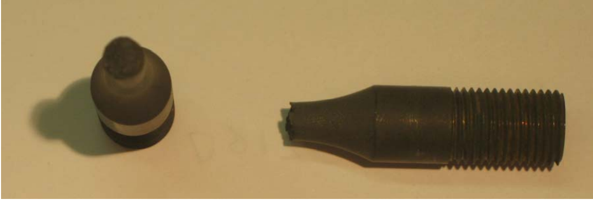
Figure A.24. Photograph of fractured specimen D912-15, 850°C test temp and 0.136 norm. strain range.
