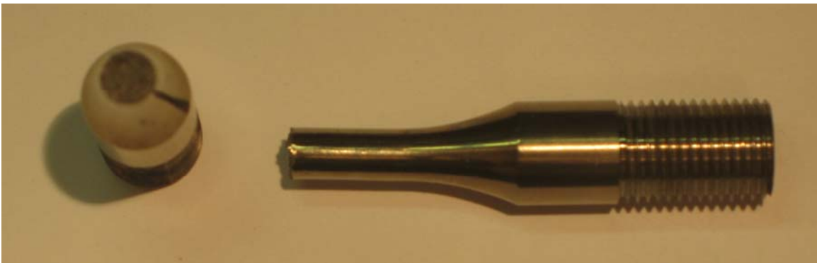
Figure A.19. Photograph of fractured specimen D912-2, 400°C test temp and 0.222 norm. strain range.
