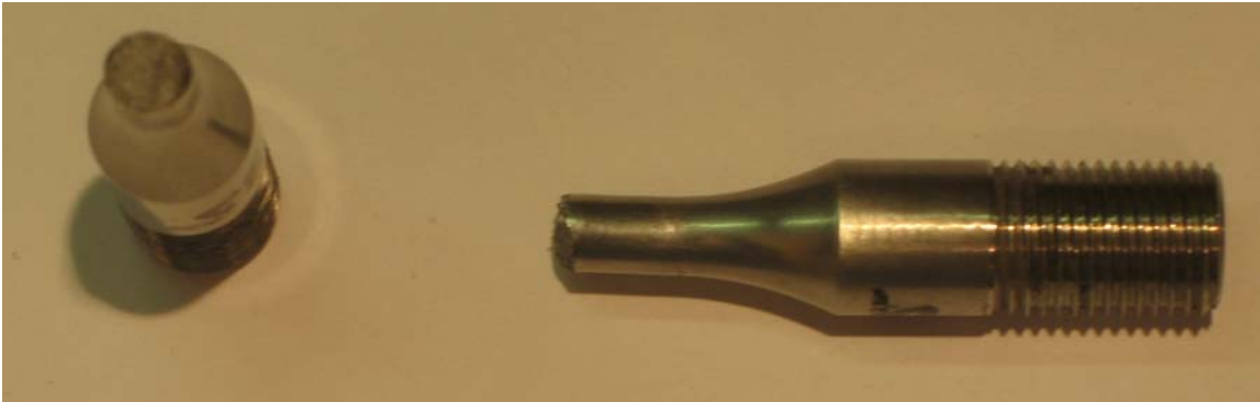
Figure A.12. Photograph of fractured specimen D912-35, 24°C test temp and 0.147 norm. strain range.
