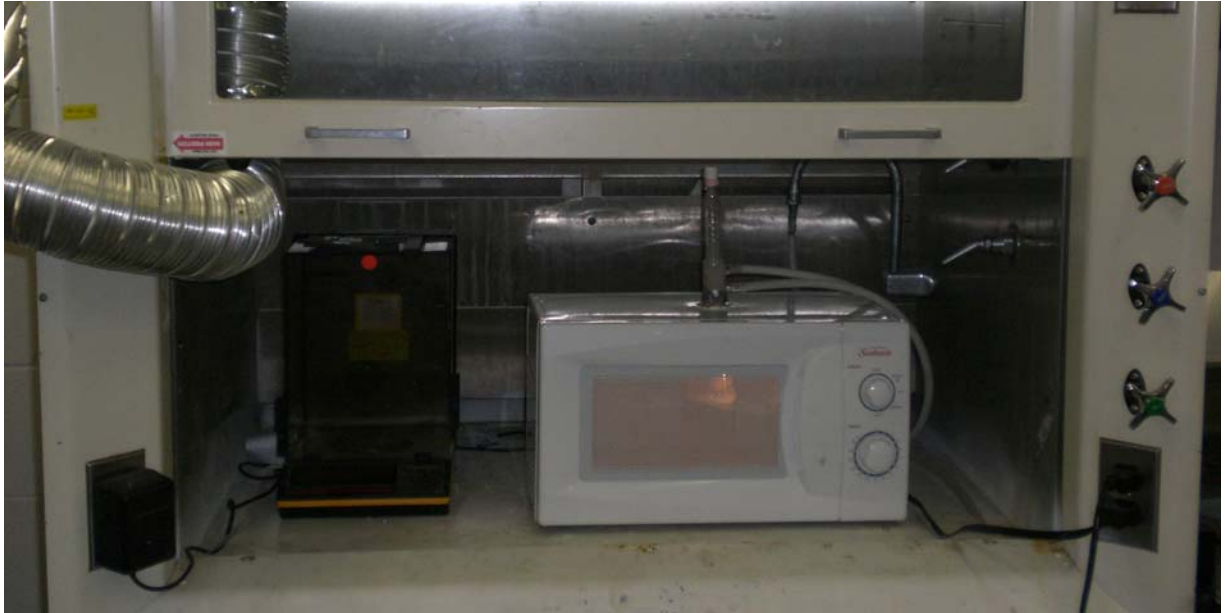
Figure 5: Set up showing microwave sythesis of HAp nanopowder
