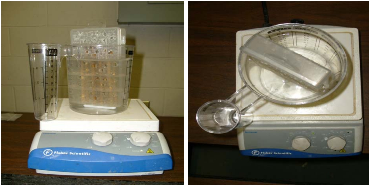
Figure 23: Experimental setup for biodegradability study of \text{TiO}_2 sample sintered at 1400^{\circ}\text{C} .
