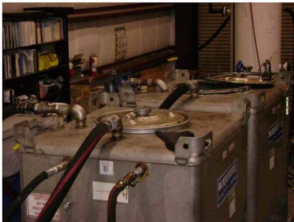
**Figure 13. Stainless steel 550gal tanks with petroleum-rated hoses**
