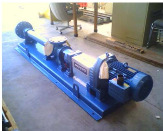
**Figure 10. Multi-Phase Pump 4-stage, 15HP**
