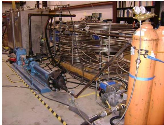
**Figure 8. Core of the loop: 300m of stainless steel tubing**
