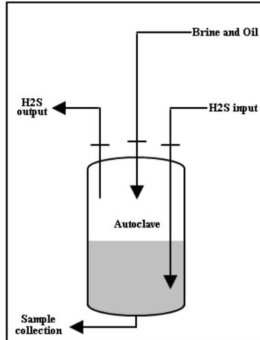
**Figure 2: Autoclave Schematic**
