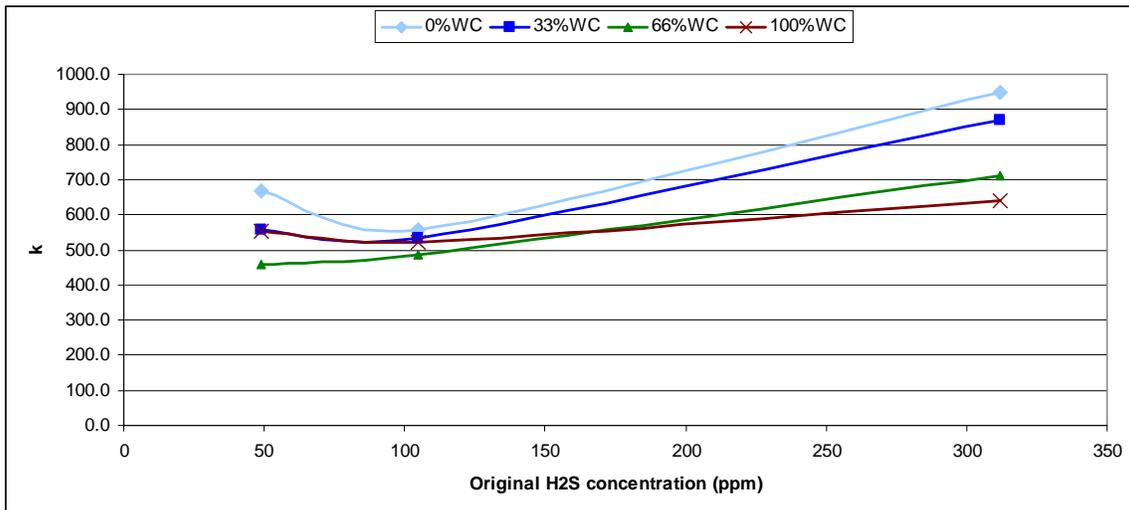
**Figure 38: Results at 70atm - Comparison of  $k$  as a function of H<sub>2</sub>S concentration**
