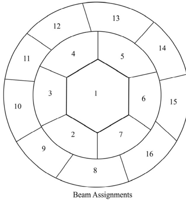
**Figure 2 S-Band Beam Pattern (View from Satellite looking at Earth Nadir) [19]**
