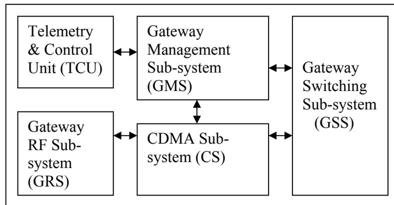
**Figure 4 Components of the Globalstar Gateway [19]**
