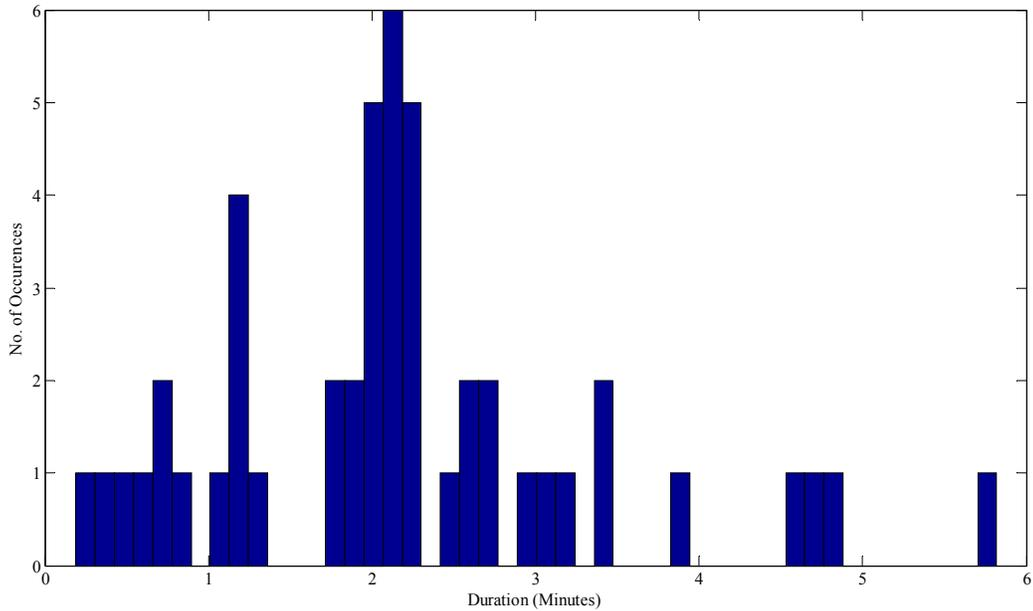
**Figure 21 Access Time for a user satellite (600 km, 90°) communicating to ground stations using Globalstar**
