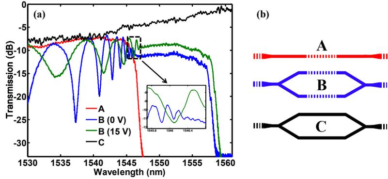
Fig. 2. (a) Transmission spectra of non-MZI grating waveguides (case A), MZI with grating at two different biases (case B), and MZI device without any gratings (case C); (b) Schematics of the three device cases in (a).
