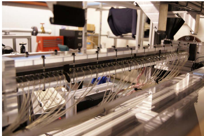
Figure 2.29: Pressure Measurement Test Section with Pressure Taps Installed
