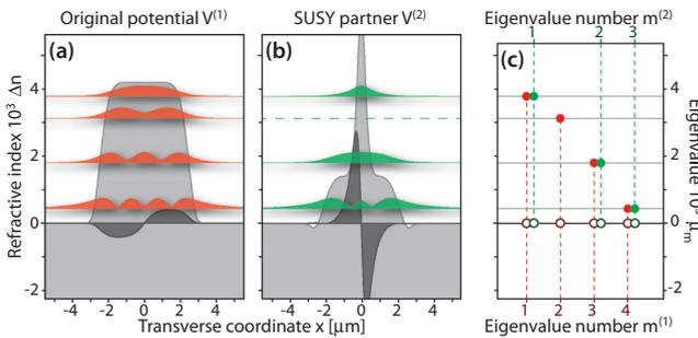
FIG. 2. (Color online) (a) Refractive index profile of a  $\mathcal{PT}$ -symmetric multimode waveguide supporting a total of four bound states, as in Fig. 1. (b) Corresponding SUSY partner where the second mode has been removed from the original waveguide. (c) Eigenvalue spectra of the two structures.
