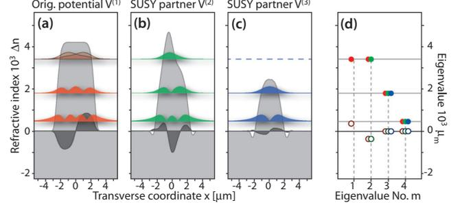
FIG. 4. (Color online) (a) Refractive index profile of a multimode waveguide supporting a total of four bound states. Here, the imaginary contrast was increased to  $\gamma = 0.2$  to induce a spontaneous  $\mathcal{PT}$ -symmetry breaking in the two lowest modes. Sequentially removing (b) the lossy and (c) the amplified modes by means of SUSY restores  $\mathcal{PT}$  symmetry in (d) the resulting structure.
