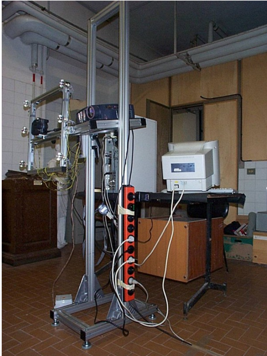
Figure 2.1: A low cost structured light 3D scanner [70].
