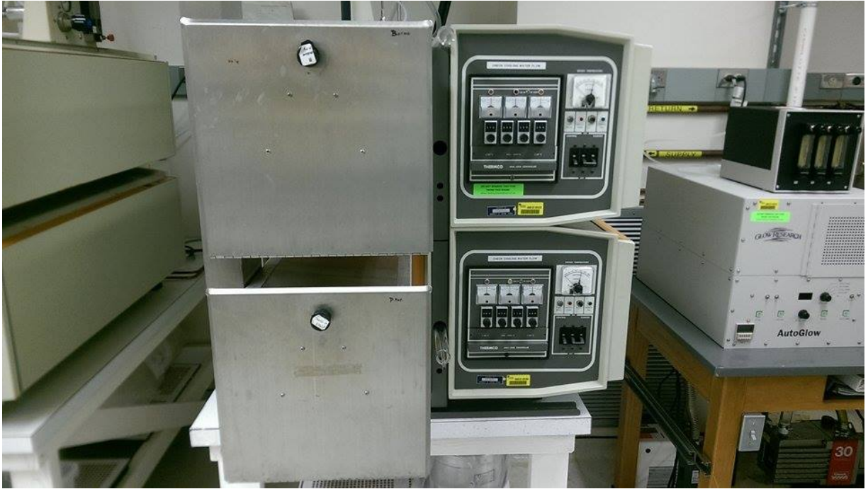
Figure A.1: Oxidation and Diffusion Furnaces
