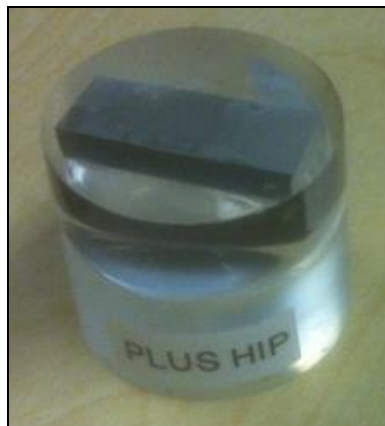
Figure 30: Mounted Cast + HIP sample prior to polishing
