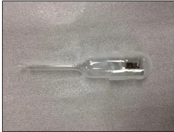
Figure 22: Typical image of one of the six as-cast samples that were encapsulated in glass tubes
