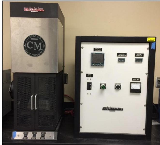
Figure 25: CM 1710 rapid high temperature (1700°C) furnace with vertical cycling capability
