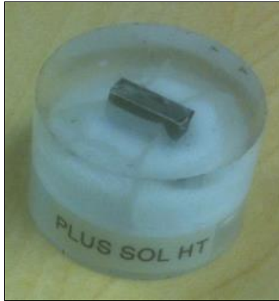
Figure 31: Mounted Cast + HIP + Solution Heat Treated sample prior to polishing
