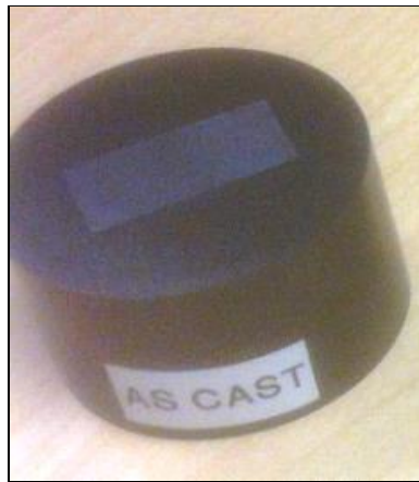
Figure 29: Mounted as cast sample prior to polishing
