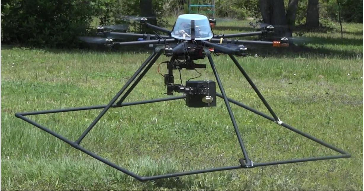
Figure 2.1.2 Octorotor platform
