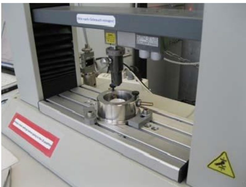
Figure 28. Photograph of the actual instrument used to carry out the ring-on-ring testing [105, 108]
