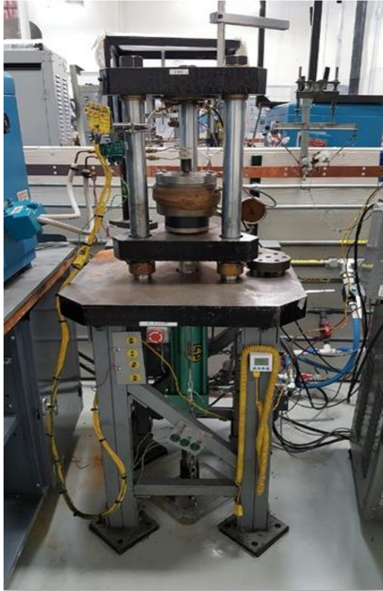
Figure 3-3: Experimental set-up for fatigue testing.
