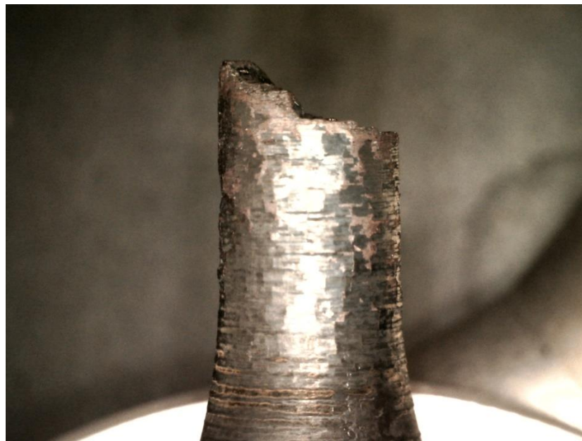
Figure A- 19. Pictures of deformed specimen BR35.
