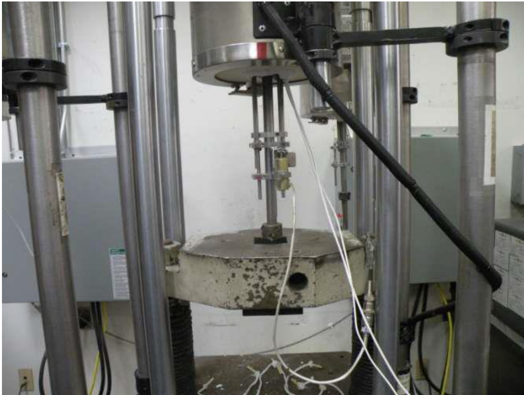
Figure 3-2: Experimental set-up for tensile testing.
