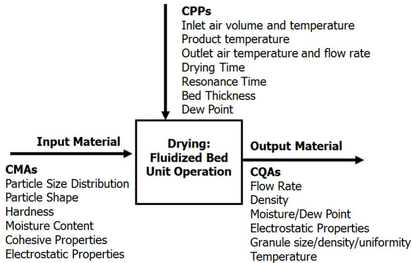
Figure 1: Block Flow Diagram a fluidized bed unit of operation and identification of possible CMAs, CPPs, and CQA
